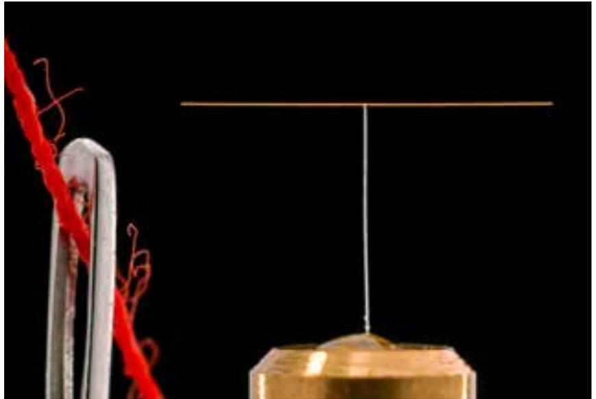
*Thin wire target. The top wire is made from gold and is 20 microns in diameter (about a quarter the width of a human hair). (A micron is  $10^{-6}$ , or one millionth of a metre.) One end of the gold wire has been polished to sub-micron smoothness, 2005. (05EC4316A)*
