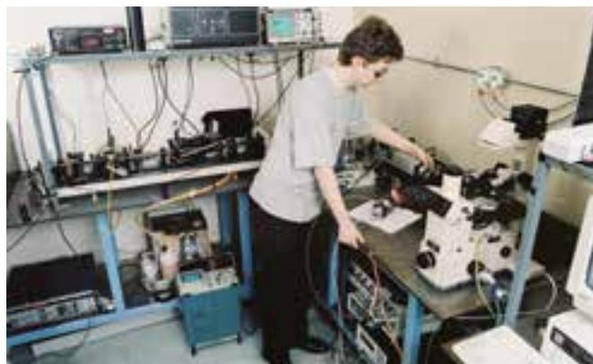
*Kevin Henbest in the Laser Microscopy Laboratory, c.1997. A Gated Image Intensifier (GOI) camera can be seen on the bench to the left of the white confocal microscope; in the background is the "cavity dumper" laser.*
