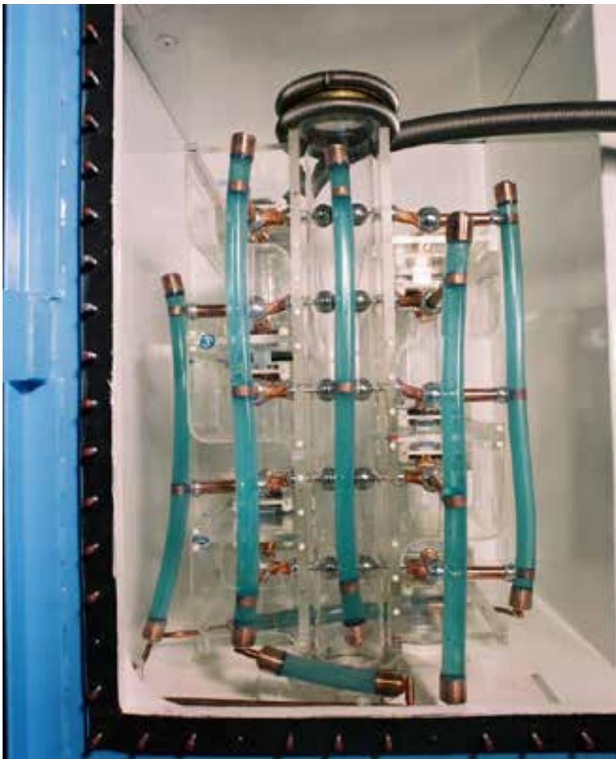
*End view of a Marx bank generator with the access panel removed, showing spark-gap column and charging resistor tubes filled with a turquoise copper sulphate solution, 1978. (27812)*
