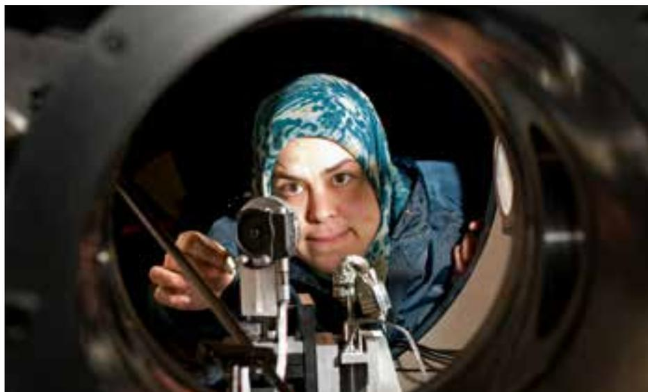
*Setting-up optics in a Target Chamber. (08EC4263)*
