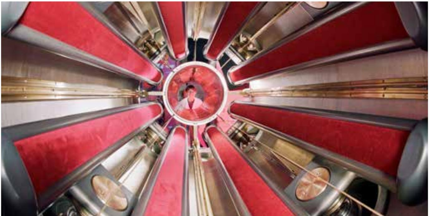
*Sally-Ann Brind looking down the barrel of the vacuum vessel. The red panels are the cathodes of the electron guns, and are made of actual velvet, which acts as a good electron emitter because its fine hairs enhance the electric field, 1994. (94RC2911)*
