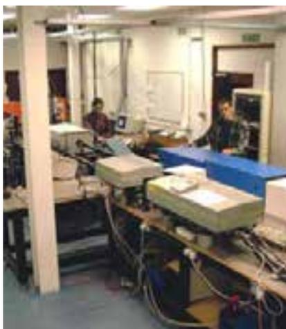
Laser Loan Pool dye lasers on the Cinétique de Réaction en Ecoulement Supersonique Uniforme (CRESU) apparatus at Birmingham University, 1998. It was expected that molecules would become dormant when cooled to 15 degrees Kelvin. This experiment demonstrated that this was not actually the case, and therefore that it was theoretically possible for water on meteors in space to perform chemical reactions.
