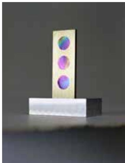
*Formvar (a type of plastic) foils on a three-target holder. Even in the early days, thin foil targets were in demand although not in the quantities required for microspheres. (23199)*
