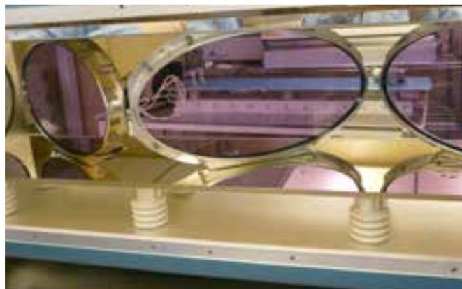
*Vulcan disc amplifiers. These are arranged in a zigzag formation at Brewster's angle to the beam in order to minimise reflection losses from the surfaces. They are purple in colour because of the neodymium "doping" (contained) in the glass which converts the energy from the flash-lamps into laser light.*
