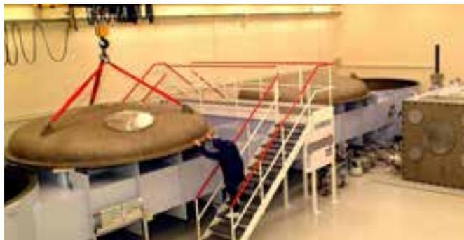
Three-section compression chamber. The “shipping container” target chamber (right) is made of 125 mm thick mild steel, is 5m x 3m x 2m in size, and weighs 60 tons. It is now surrounded by 100 tons of lead (about half of which was supplied by the ISIS facility), 50 tons of concrete, and 20mm thick aluminium plates, 2002. (02EC1630)
