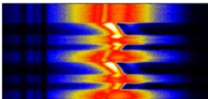
*This image illustrates how molecular catalysts work. These molecules in solution are designed to break down CO<sub>2</sub> on electrode surfaces; ULTRA is able to distinguish between the very small number of molecules that happen to be at the electrode's surface, and the overwhelmingly large number of molecules swimming freely in solution.*
