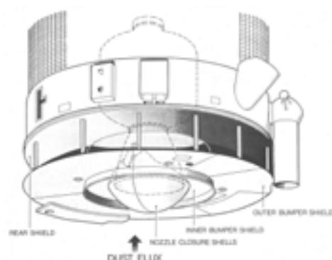
*The DIDSY instrument was tested and calibrated in various ways, one of which was by firing pulsed laser beams at the dust shield. The energy and duration of a laser shot were similar to those of a small dust particle impacting the shield.*
