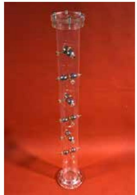
*A studio portrait of a Marx spark-gap column; in reality this was about 1.5m in height. The pairs of stainless steel electrodes are the switches that connect the Marx capacitors when the machine is fired. (27554)*
