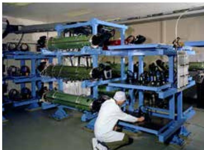
*A picture of the "main 6" 108mm diameter amplifiers in the Vulcan Laser Area, 1983. (83FC1737)*
