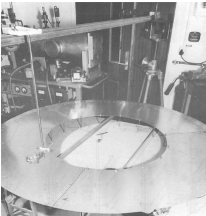
*The Dust Impact Detection System (DIDSY) on the Giotto spacecraft was designed both to protect it from impacts of cometary dust particles moving at around 60,000 mph, and to measure the number and sizes of those impacts as the probe flew through the tail of Halley's comet.*
