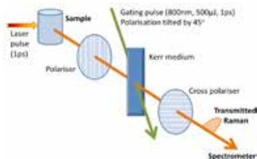
In 1993 the TR<sup>3</sup> Spectroscopy Facility was enhanced by the introduction of an optical technique known as the Kerr gated Raman collection system. The Kerr medium acts as an optical shutter, and enabled scientists to observe for the first time very faint Raman signals emitted by samples which would otherwise have been swamped by the much stronger fluorescence signals.
