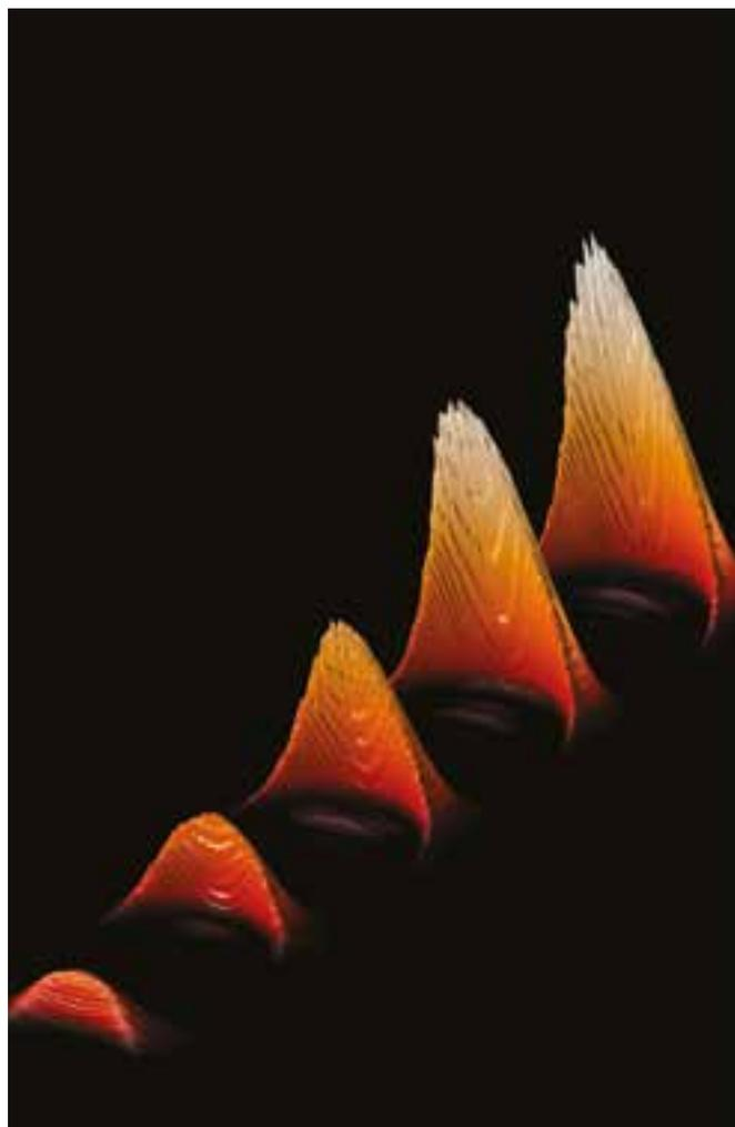
*A computer simulation of a sequence of snapshots of the growing pulse in a Raman amplifier, showing that the pulse can be amplified while its envelope remains smooth.*
