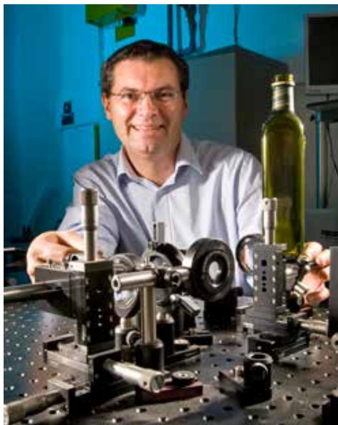
SORS can also be used to analyse the contents of bottles to determine whether they contain a harmless liquid such as milk, cosmetics or medicines, or a dangerous chemical such as acid or explosives.
