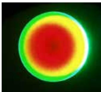
Image generated by an OPA laser in the 1990's. This light pulse is only 100 femtoseconds long (a femtosecond is  $10^{-15}$  seconds) so can capture snapshots of molecular reactions as they occur.
