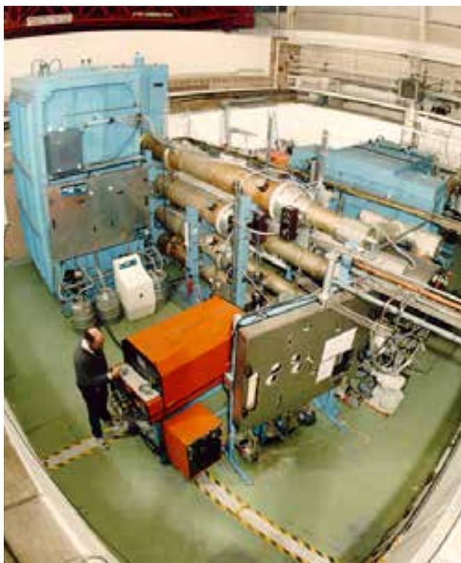
*Graeme Hirst in the Titania laser bay in R2 adjusting the trigger laser. The orange box was a small KrF laser, the beam of which was used to trigger spark-gaps for switching the high-voltage pulses in the Titania machine. The tall blue cabinet at the back is a Marx bank.*
