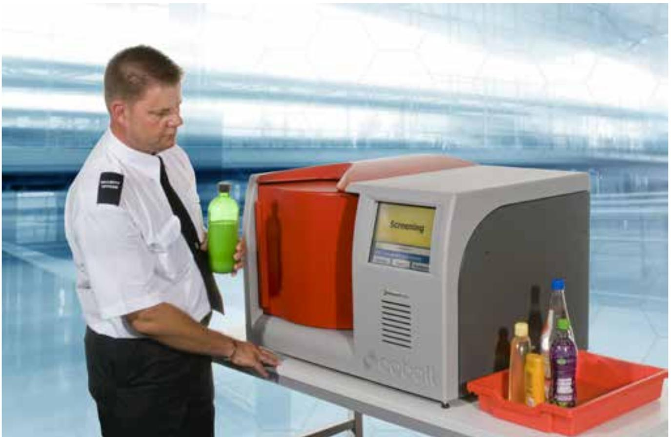
*Work on SORS techniques has led to the development of the Insight100 machine, a bottled liquid screener for use in airports. This was developed and marketed by an STFC spin-out company Cobalt Light Systems Ltd. There are about 400 operational units in 70 airports across Europe and Asia; Heathrow alone has over 80. It is hoped that this technology will allow the relaxation of airline restrictions on bringing liquids on board aircraft.*
