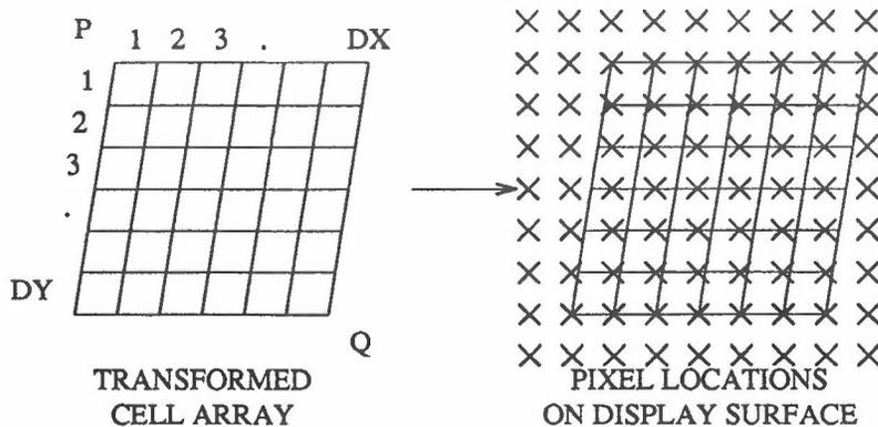
**Figure 11 - Mapping CELL ARRAY cells onto pixels**
