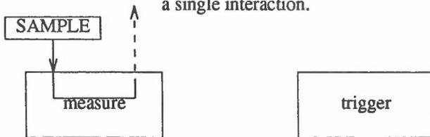
EVENT mode Value and device identification sent to single queue on trigger firing and removed by a call to AWAIT EVENT.
