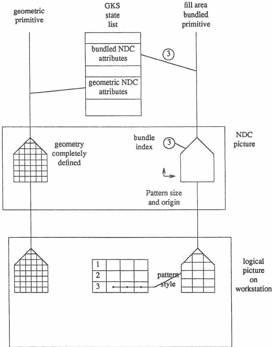
Figure 6 - Attribute binding for primitives
