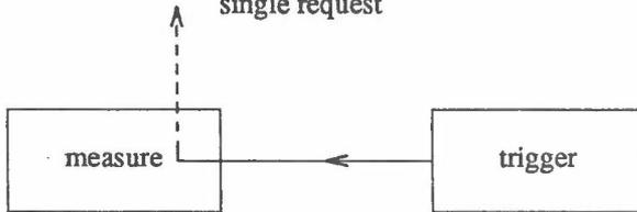
SAMPLE mode Trigger inoperative. Value returned for each call to SAMPLE. Multiple calls to SAMPLE in a single interaction.
