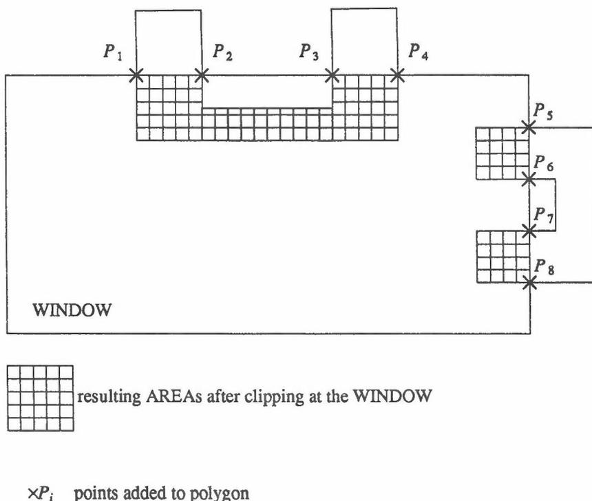
Figure 4 - Examples of FILL AREA clipping
