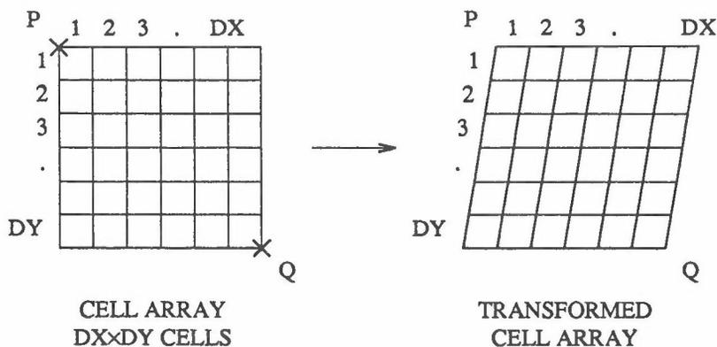
Figure 5 - Mapping of CELL ARRAYS
