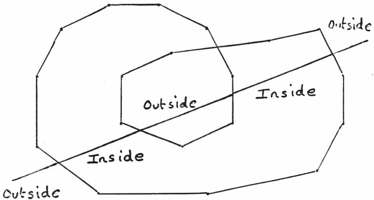
Point is inside boundary if arbitrary point at infinity has a line from it which intersects the boundary an odd number of times
