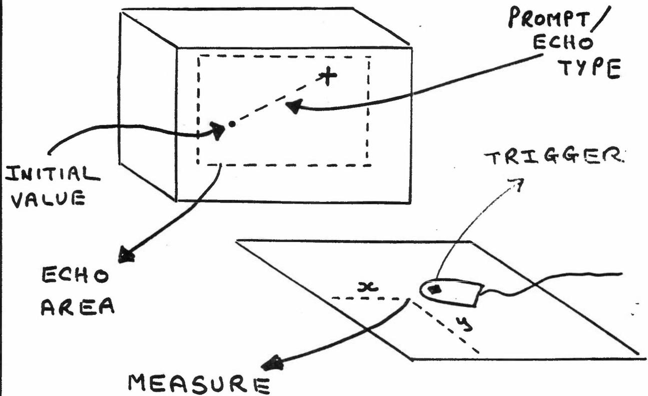
**MEASURE** value determined by one or more physical input devices. Can be thought of as a process independent process that sends a message to one or more Logical Input Devices
