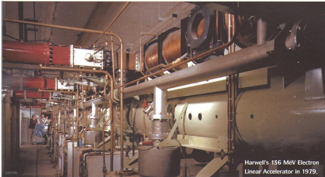
Fig. 2. The Harwell 136 MeV electron linac, inside the linac hall, looking upstream<sup>6</sup>.
