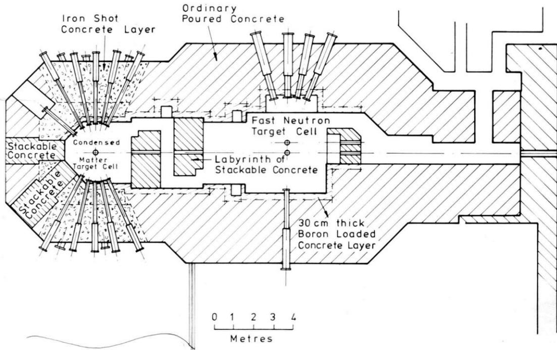
Fig. A1. More detailed drawing of the Fast Neutron Target (FNT) Cell and the Condensed Matter Target (CMT) Cell and their respective neutron flight paths. The axis of the 136 MeV linac was located above the axis of the older 1959 ~50 MeV linac so that flight paths from the FNT and CMT would not foul the flight paths from the Neutron Booster Target (NBT).
