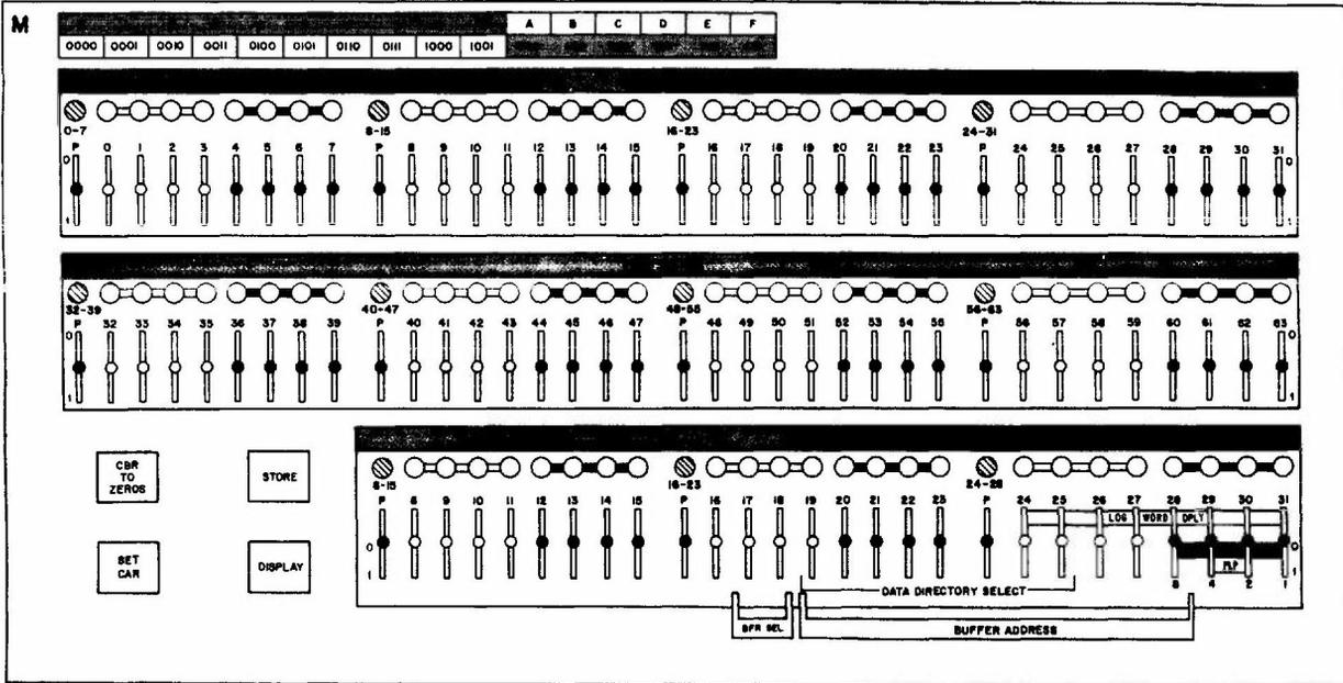
The address switches have locking set positions. The associated bit position of the console address register is set according to the position of the switch when the SET CAR key is pressed. (When this switch is down, the bit position is set to 1; in the center position, the bit position is set to 0.) The console address register addresses storage or a register as specified by the address compare, CRT display and tape operation, or store/display/storage select switches.
