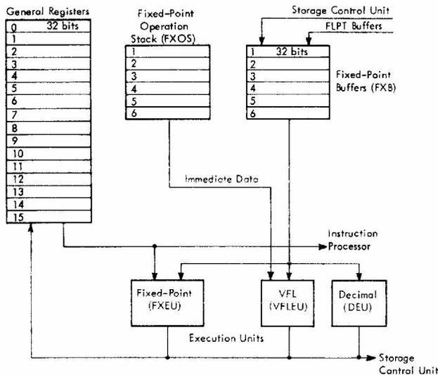
Figure 7. Fixed-Point/VFL/Decimal Execution Element
