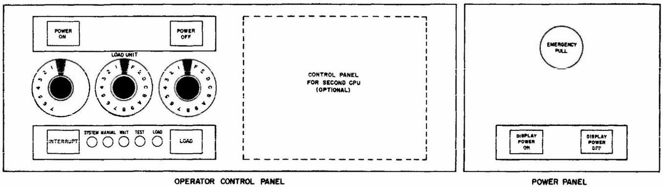
Figure 10. Operator Control Panel and Power Panel
