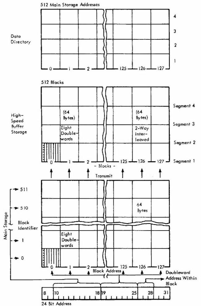
Figure 5. High Speed Buffer Storage
