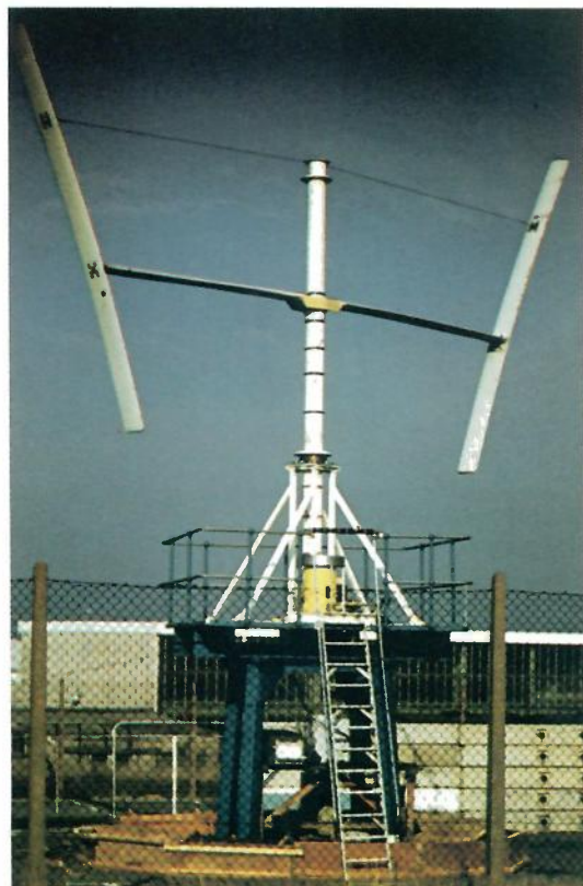
A 6.5 kilowatt aerogenerator built at Chilton for Cambridge University.
