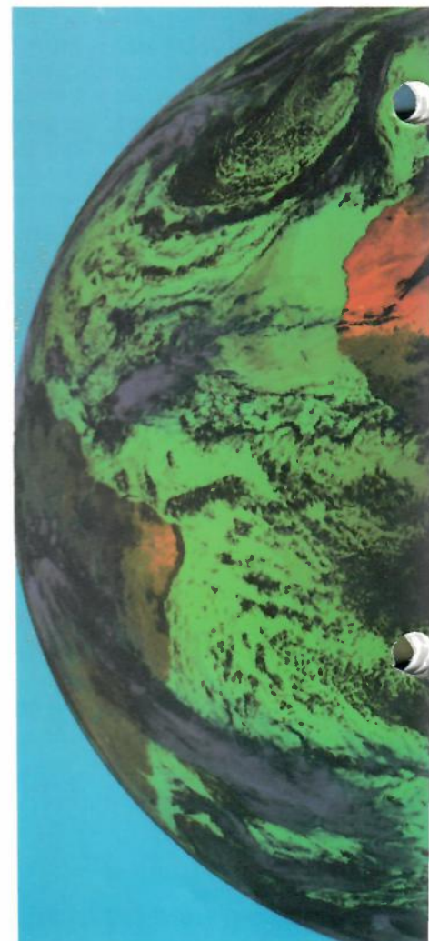
A coloured Meteosat image of the Earth produced by the Interactive Planetary Image Processing System at University College, London. The green shows the "visible" image, red is infra-red radiation and blue is water vapour (Photo: UCL).
