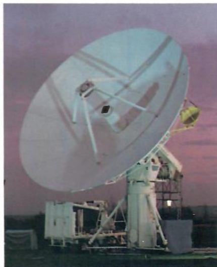
The 12m diameter antenna which is being set up to track the Infra-Red Astronomical Satellite.
