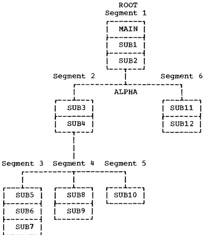
Figure III-8. Overlay Tree Structure Having Six Segments
