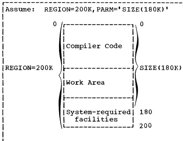
Figure III-3. Storage Structure Using SIZE and REGION
