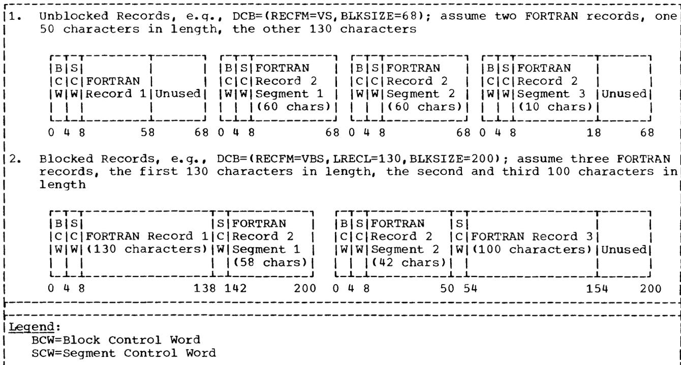
Figure I-23. EBCDIC Sequential Data Sets--Structure of Unformatted Records
