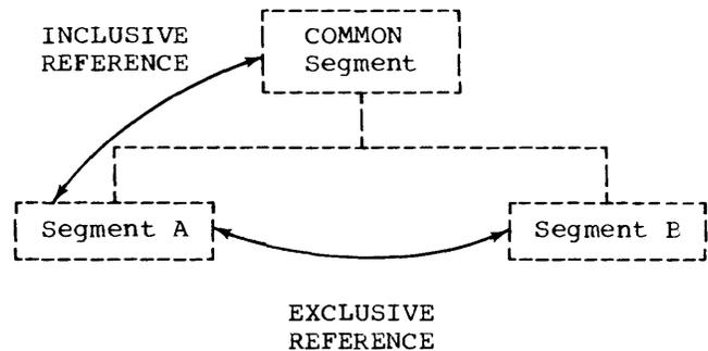
Figure III-11. Communication Between Overlay Segment
