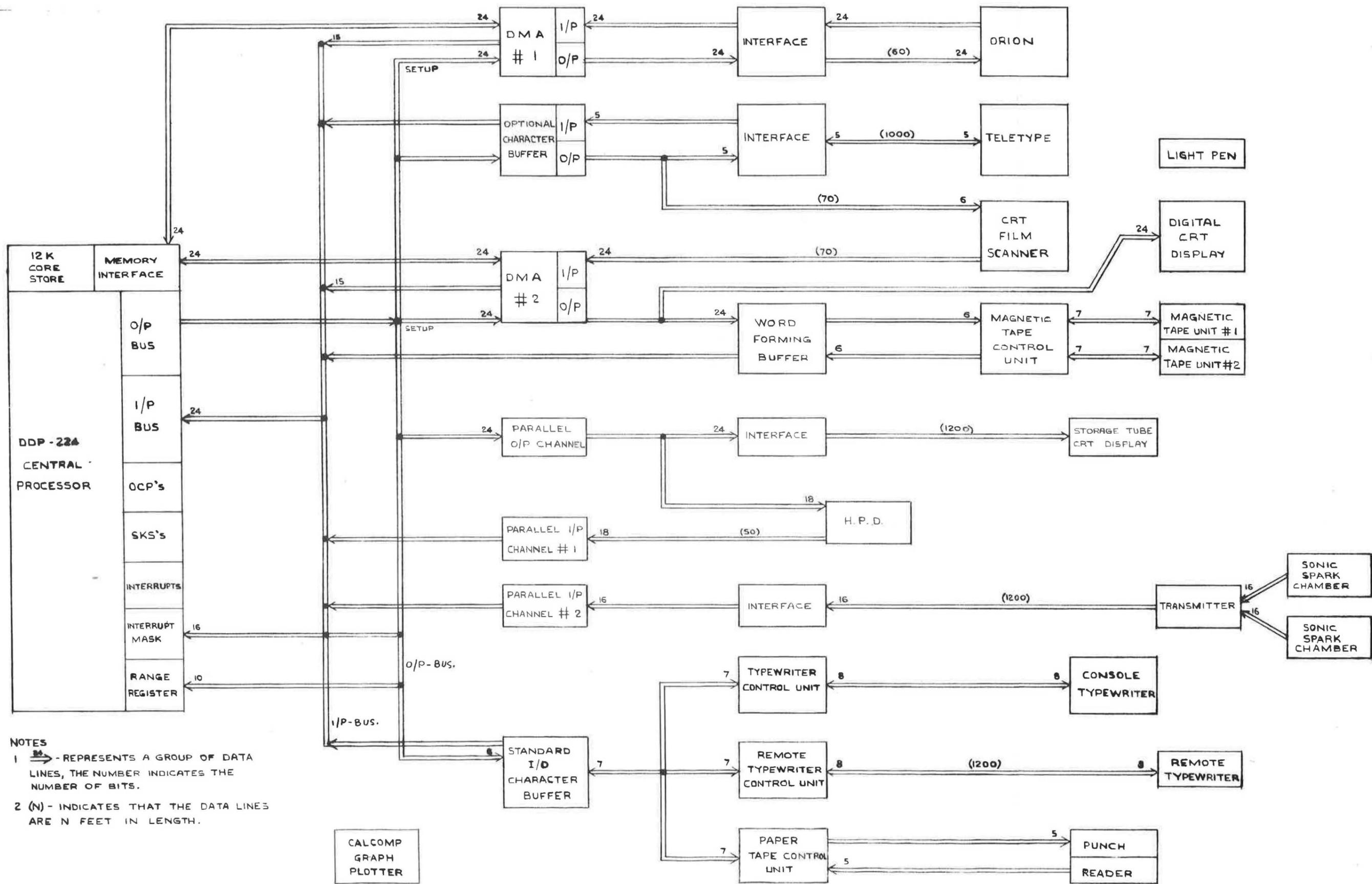
Fig. 1 DATA FLOW BETWEEN THE CENTRAL PROCESSOR CHANNELS AND DEVICES
