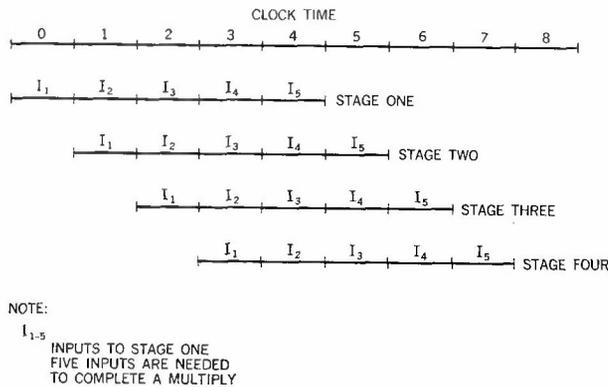
Figure 15 Timing diagram for abstracted iterative hardware.
