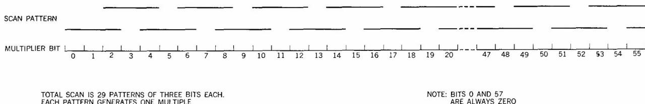
**Figure 8** Scanning pattern for multiplier.
