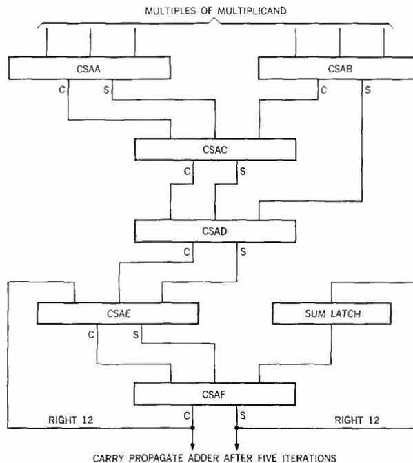
Figure 13 CSA tree with accumulating loop at output.
