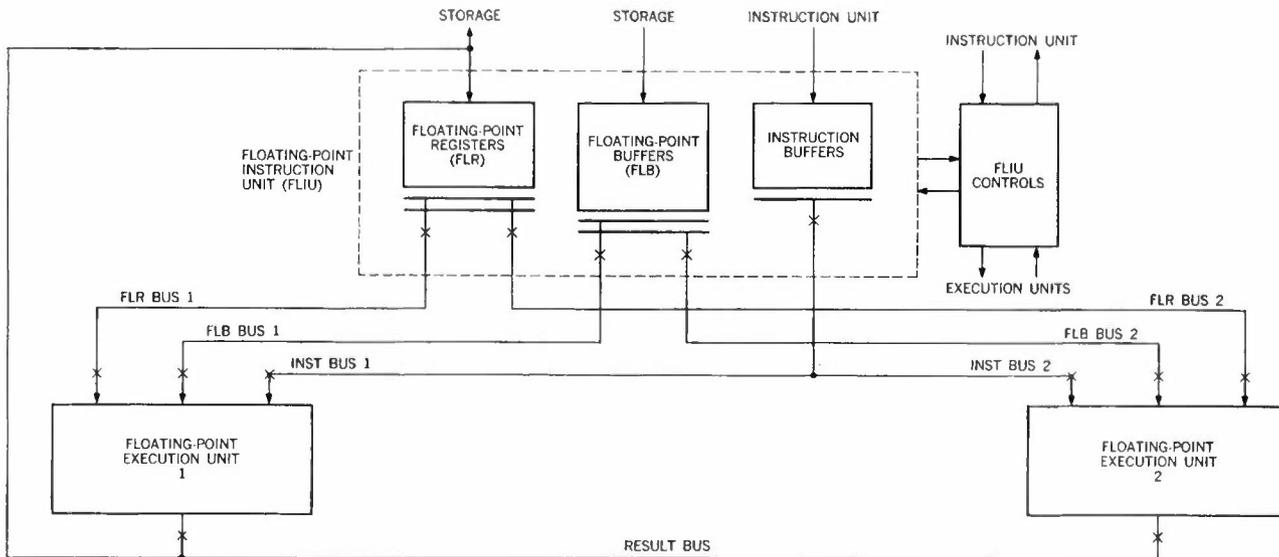
Figure 1 Floating-point execution unit capable of concurrent execution.
