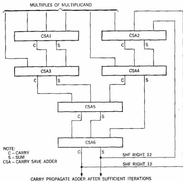
Figure 12 CSA tree with feedback loop from output.
