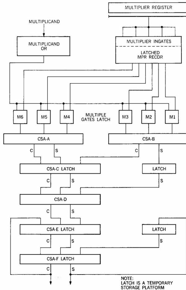
Figure 16 Multiply iterative loop showing temporary storage.
