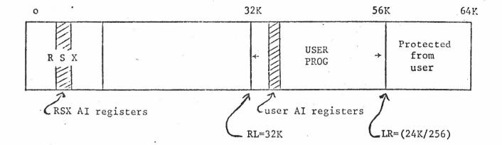
User physical area 32K - 56K User address space 0 - 24K Relocation register 32K Boundary register 24K/256 (number of 256 words in prog)
