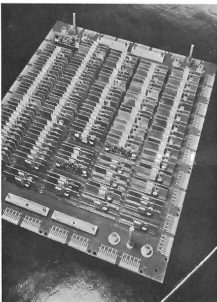
3 12-layer platter loaded with circuit modules
