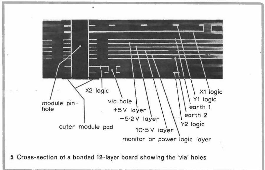
5 Cross-section of a bonded 12-layer board showing the 'via' holes
