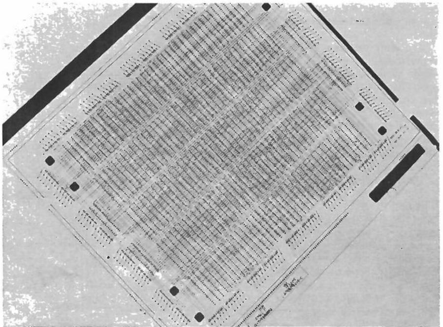
4 Pair of logic layers for carrying signals between modules inside the platter
