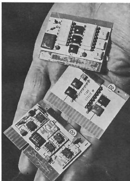
2 Unencapsulated integrated-circuit modules using special Motorola e.c.l. on single silicon chips
