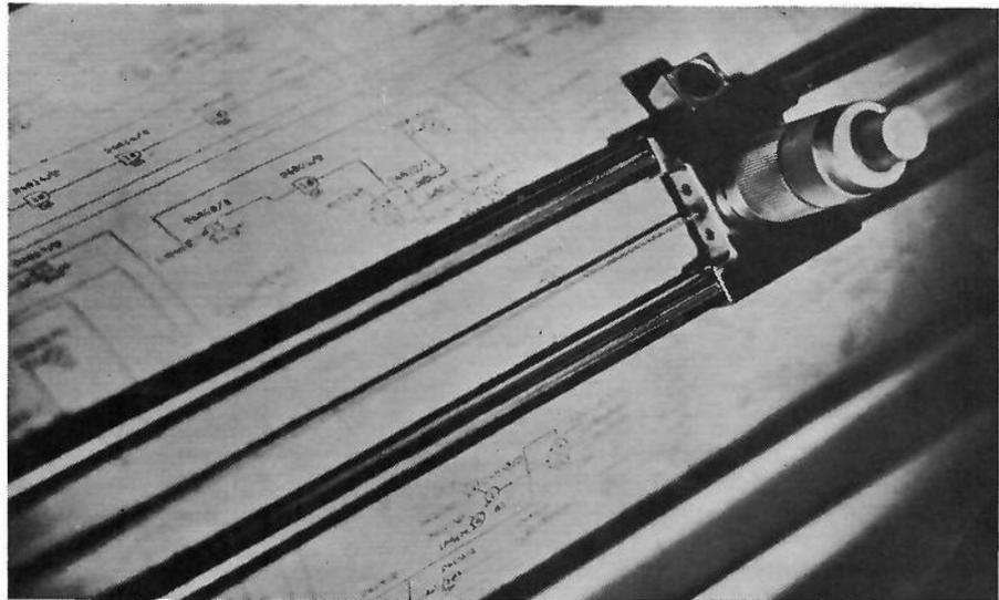
9 Calcomp plotter drawing a logic diagram online from a computer
