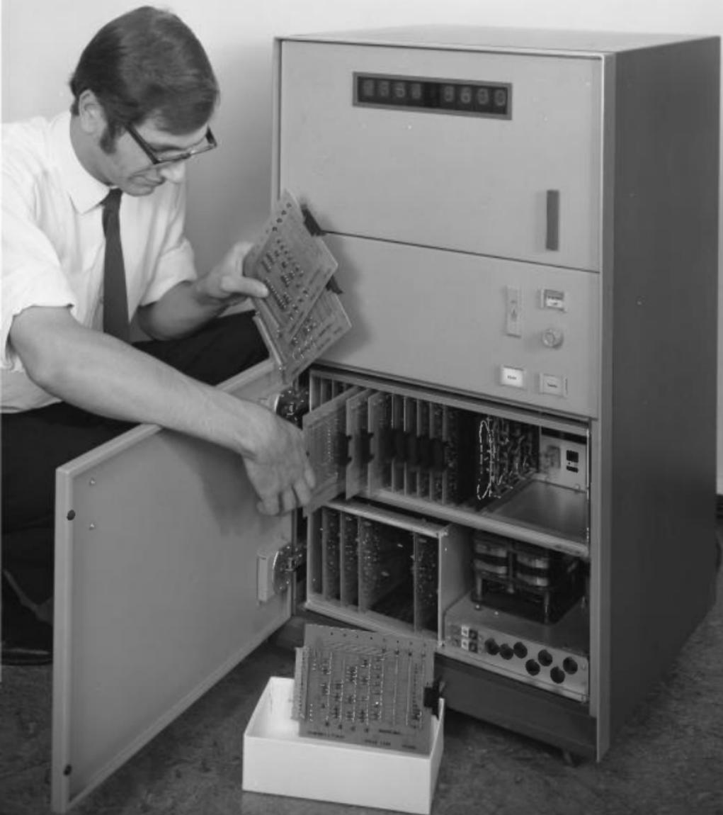
1.1.3.6. Three types of paper tape are available, ie Ferranti 5-track, Ferranti 7-track and ICT 1900 tape. Associated with each type of paper tape is a set of three circuit boards marked Board No 1, 2 and 3. These boards should be changed over when necessary as indicated in figure 5. Here, Board No 1 for 7-track tape is being removed while Boards 2 and 3 are shown partially withdrawn.
