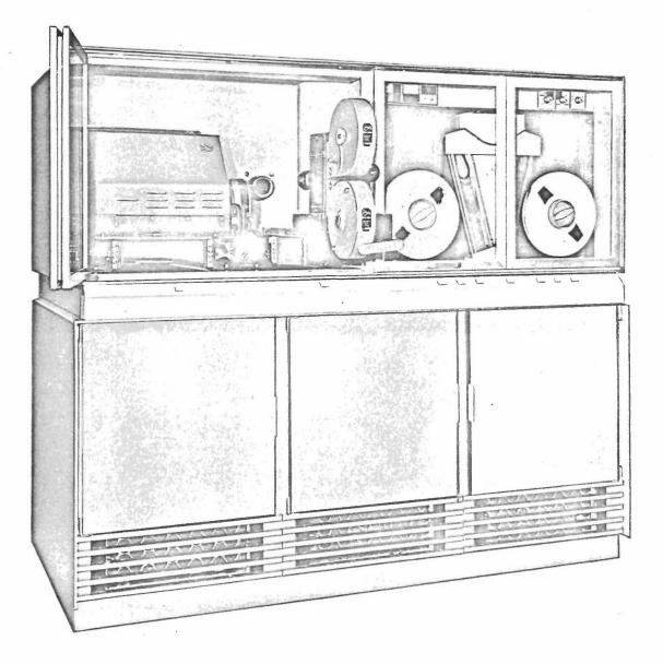
Figure 2. B-L 120, Microfilm Camera Pulled Forward for Loading
