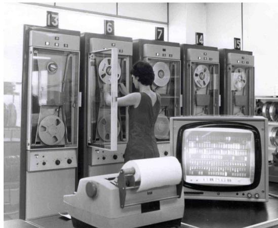
Eileen Perkins loads one of Ampex magnetic tapes in the Atlas Operations Room; in the foreground is a teletype printer and a CCTV image of the Engineer's console downstairs, 1968
