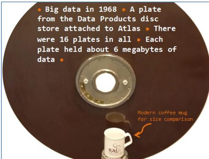
• Big data in 1968 • A plate from the Data Products disc store attached to Atlas • There were 16 plates in all • Each plate held about 6 megabytes of data •
