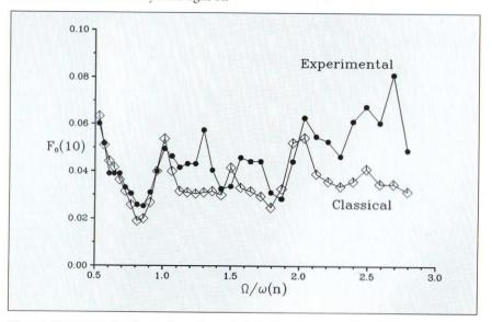
Figure 3: Graph comparing the experimental,  $\bullet$ , and classical,  $\Diamond$ , microwave field amplitudes needed to produce 10% ionisation for low scaled frequencies.
