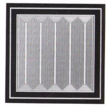
Figure 2: The surface of a silicon drift photodiode opposite the photosensitive side. The detector is divided into five cells with an n-type anode, at the centre of each cell, surrounded by field shaping p-type cathodes. Electrons drift within the wafer up to 1 mm to the anode. The total area of the detector is 15mm x 15mm.
