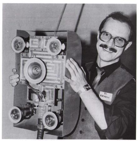
Dr Rachkov of the Institute for Problems in Mechanics demonstrates a wall-climbing robot designed for the inspection and maintenance of buildings.
