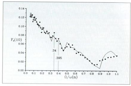
Figure 2: Graph comparing the experimental, •, and classical, solid line, microwave field amplitudes needed to produce 10% ionisation for scaled frequencies smaller than unity. The experimental points nearest to the 1/3 and 2/5 resonances are seen to be locally more stable.
