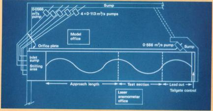
Meandering river with flood plain configuration of the flood channel facility. (Pictures: Hydraulics Research Ltd).
