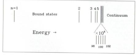
Figure 1: Energy levels of low- and high-states of atomic hydrogen, showing the increasing density of states with increasing principal quantum number, n
