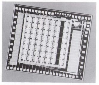
Figure 4: The prototype pixel amplifier chip. It contains 56 identical cells 300µm x 300µm. A full-size version will be bump-bonded to a detector diode array.
