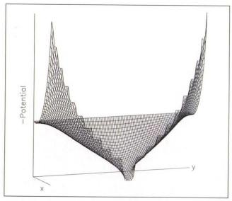
Figure 3: The electric potential distribution in one cell of the photodiode shown in figure 2. Electrons follow the path of steepest descent to the anode.
