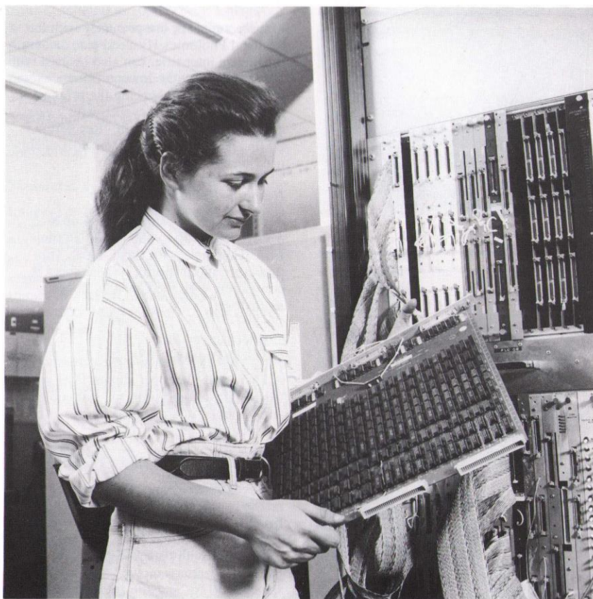
Visual inspection of a completed board for use in an experiment at CERN. The board utilises both commercially available and custom-designed chips and was produced in the Electronics Division Workshops at Rutherford Appleton Laboratory. The board was also designed at RAL, using the advanced board layout CAD programmes that the Electronics Division has recently acquired.
