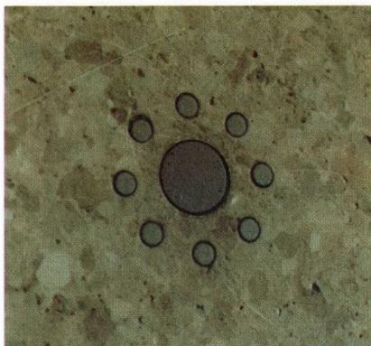
Miniature voltammetric carbon electrode on-line monitoring (photo: UMIST).
