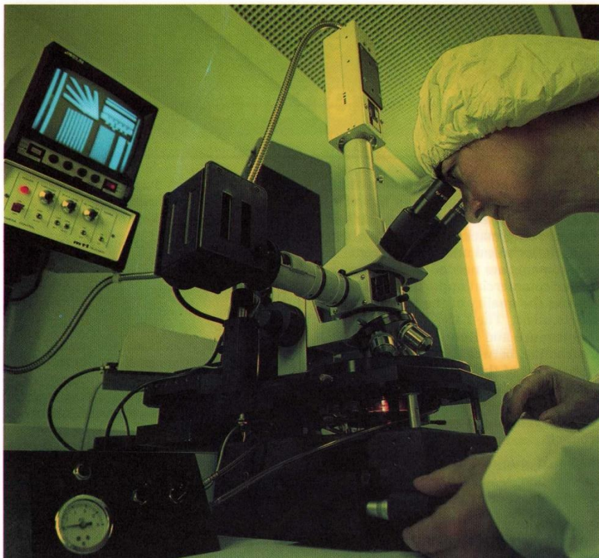
An operator using a mask aligner for device fabrication (photo: Glasgow University).
