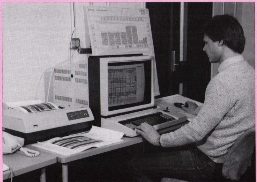
VLSI design workstation with graphics terminal, data tablet and colour plotter.
