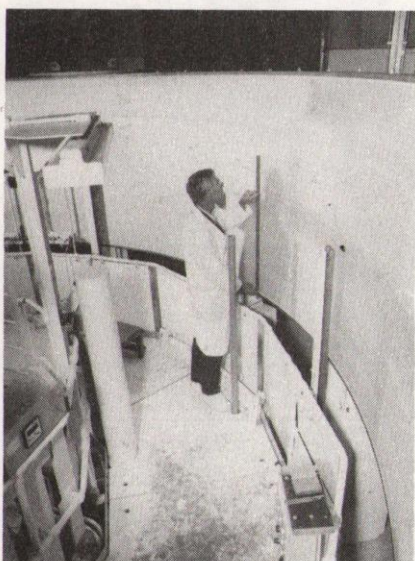
86RC 4630. Measuring the pitching of the 296 turns wound in a main coil module.
