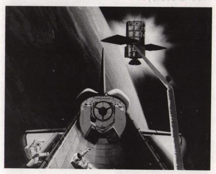
The astronaut's attempts to capture Solar Max were abandoned and the spacecraft heaters were switched off to conserve battery power. Solar Max's magneto-torquers were then used to point Solar Max at the Sun once more and to put it in an attitude which would allow capture by the Shuttle's remote manipulator arm. Fortunately, this was achieved before the batteries ran flat - but only just!
