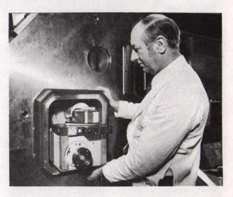
The refrigeration control vessel which was completed mechanically some months ago has now had radiation shields fitted and all exposed parts superinsulated.
