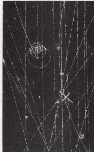
Part of the millionth bubble chamber picture measured with Birmingham University's automatic scanning machine. The event is a "601" (six charged prongs and a neutral strange particle decay) from film of a -8.25 GeV/c kaon beam into the CERN 2m hydrogen bubble chamber.
