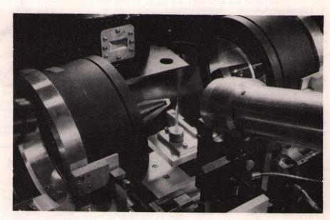
A milestone in the progress of the laser division was passed on Friday, 29 April when laser compression was recorded with the first shot of the new two beam laser at a glass microballoon target.
