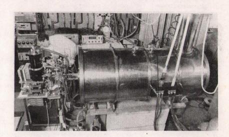
After being used in a two-week experiment by Appleton Laboratory researchers in their investigations of molecular absorbtion in the two-millimetre wavelength region as part of their research programme into atmospheric propagation, a superconducting dipole magnet designed and built at RL is being shipped to Argonne Laboratory in the US for use by an Imperial College Group in ultraviolet spectroscopy work on the diamagnetic Zeeman Effect.
