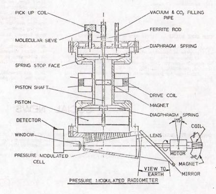
two similar PMRs to cover the full height range compared to 8 switched channels in Nimbus E covering a smaller range. The complete instrument containing two PMRs weighs 28 lbs, is 8" x 10" x 16" high and consumes 5 watts power.
