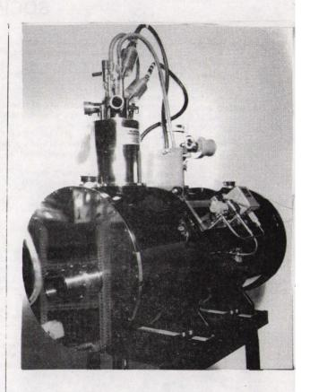
magnetic field. This enables the direction of spin of incident protons and scattered neutrons to be reversed without interruption to the experiment. A vacuum pump associated with the equipment automatically pumps the cryostat vacuum vessel if the pressure within it rises above  $10^{-5}$  Torr.
