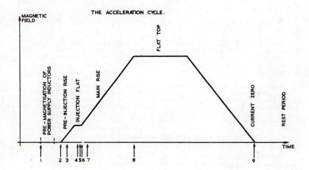
The following sequence of events makes up an acceleration cycle which can be repeated once every two seconds.
