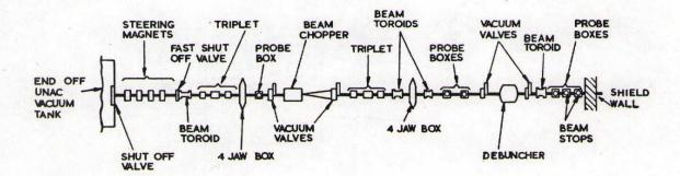
Steering Magnets: These are used to position the beam along the centre of the flight tube (aluminium pipe pumped to very low pressure).
