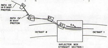
The system is designed to be 'achromatic' so that protons of slightly different energies which enter  $\mathbf{E}_1$  along the same path, will enter the synchrotron along the same path. The system can be adjusted to give a large variation in the radial position of the injected beam, while still maintaining the achromatic property. Injection takes place while the magnet field is rising. The rising field shrinks the orbit of the beam and it misses the inflector on subsequent revolutions.
