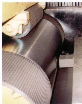
Laser in place to analyse steel sheet on rollers.
