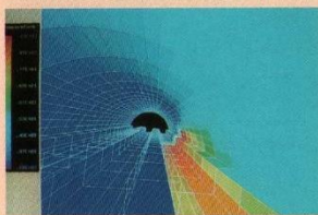
Computational Fluid Dynamics (CFD) was used to investigate the Kings Cross fire disaster and the resultant 'Harwell Trench Effect' changed the outcome of the Public Enquiry. The fireball that killed 31 people was proved to be due to chimney draught up the escalator and not to explosive combustion of paint. (HRC 46468)
