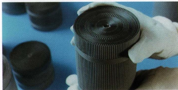
FeCrAlloy steel coated with platinum-based catalyst for car exhaust systems. (H 4817/180c)
