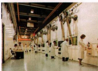
Radiochemistry on beta/gamma sources in a suite of B220 'caves'. Workers using manipulators are protected by shielding up to two metres thick. (HRC 14403)
