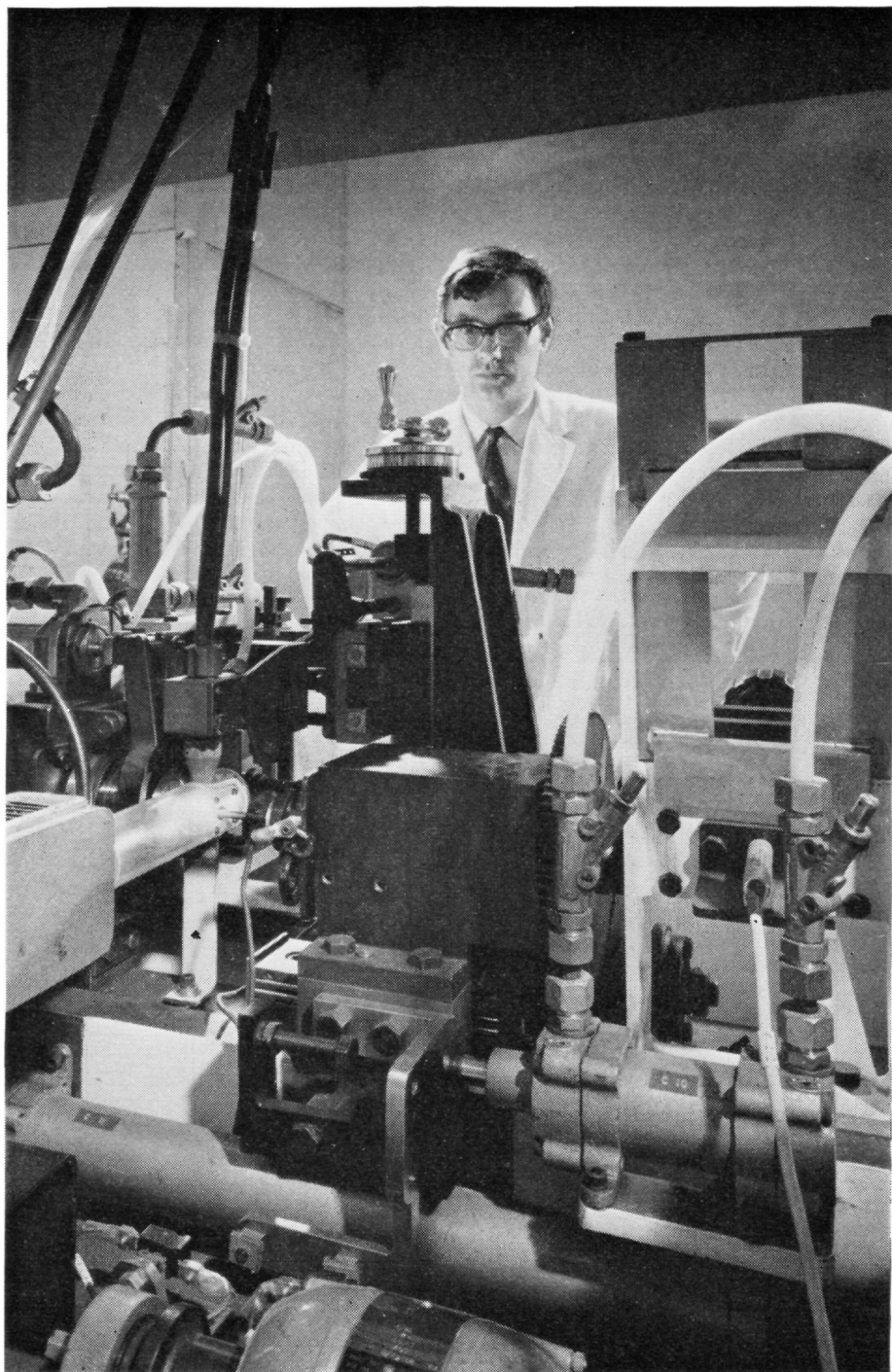
The first large-scale plant for the manufacture of plutonium enriched fuels has been built at Windscale. Initially it will make the fuel for the Dounreay Prototype Fast Reactor (P.F.R.) but will have additional capacity for reactor fuels. The plant is extensively automated and remotely controlled. The picture shows fully automated, logic controlled welding machine for end preparation of plutonium loaded P.F.R. fuel pins.
