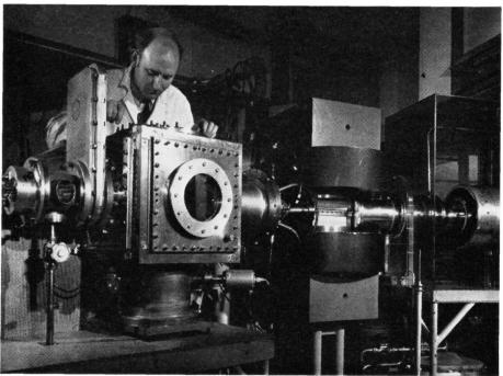
Part of the work of the Metallurgy and Electronics and Applied Physics Divisions at Harwell involves the development of techniques for injecting selected ions, including radioactive tracers, into solids, particularly semi-conductors. Observing a silicon specimen during an implantation with phosphorous ions.
