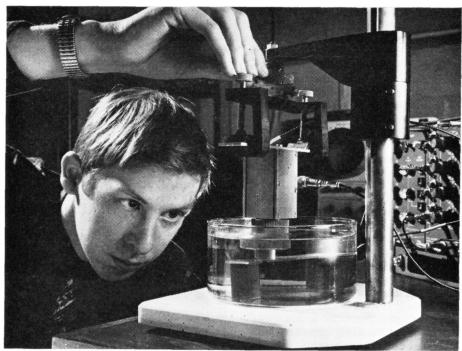
Since it was set up in 1967, the Nondestructive Testing Centre at Harwell has carried out sponsored research and development work for many industrial organisations, thus enabling them to improve quality control. Setting up a 100 MHz cadmium sulphide ultrasonic transducer to obtain reflections from a thin metal sheet.
