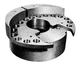
IT'S MADE OF LEAD and shows that Lead Fabricators Ltd. machine this material to fine tolerances and to a high quality of finish no matter how intricate the design. This shielding for a gate valve, part of a nuclear power station's fuel element hoist, was machined from a solid casting of 4% antimony-lead alloy. Operations included accurate boring and vertical machining of several transition radii to mate perfectly with the contour of the valve profile.
