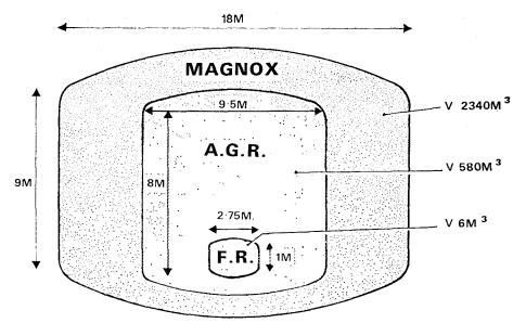
Figure 4. Core dimensions of 600 MWE reactors.
