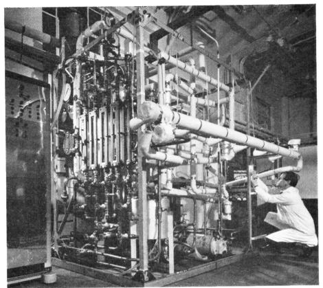
The Heat Transfer and Fluid Flow Service at Harwell uses special equipment and the special knowledge gained by the Authority in this field, to solve specific industrial problems under a confidential consultancy and testing scheme operated on a rechargeable basis. A view of two-component condensation experimental apparatus—one of many engineering rigs available for use in this service.
