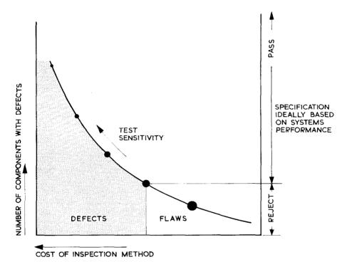
Fig. 3 Economic importance of setting a realistic specification to distinguish between harmful 'flaws' and acceptable 'defects'.
