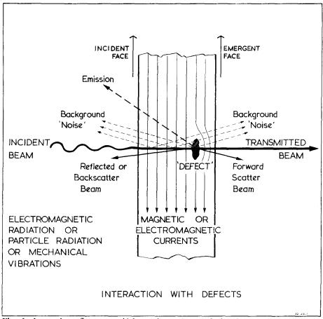
Fig. 6 Interaction effects on which nondestructive methods of internal flaw detection are based.
