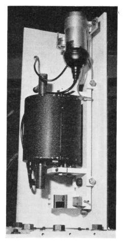
Fig. 3 Installation of the laser unit and beam shielding tube on the roof of the cell.
