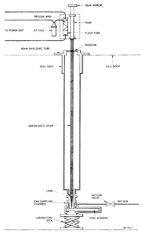
Fig. 6 Diagrammatic arrangement of the laser unit and gas sampling chamber.
