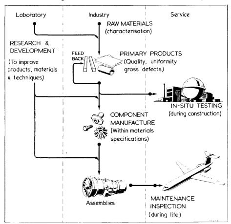
Fig. 1 Application of nondestructive testing (each black spot corresponds to an area of application)
