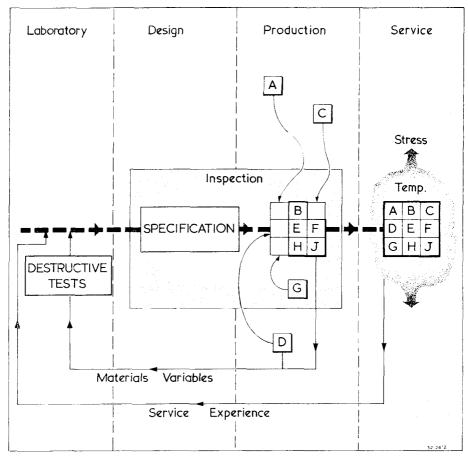
Fig. 2 Evolution of nondestructive testing techniques showing the essential information feedback loops from production and service.
