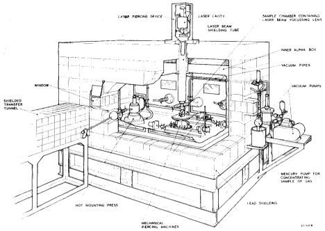
Fig. 2 Diagrammatic layout of the laser piercing equipment. The mechanical drilling equipment is also shown.
