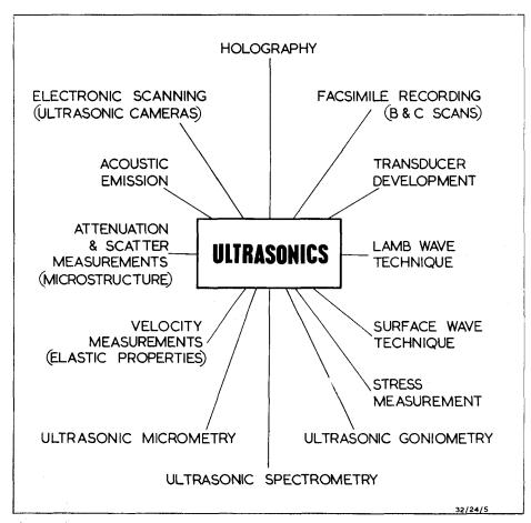
Fig. 8 Areas of current development in ultrasonics.
