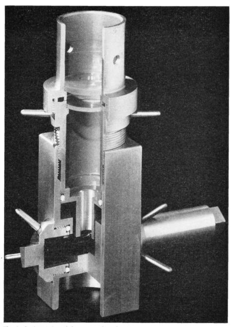
Fig. 4 Sectioned view of the gas sampling chamber.
