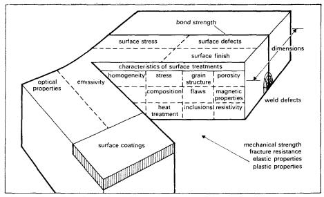
Fig. 4 Scope of non-destructive testing indicating range of materials variables that can influence mechanical strength.
