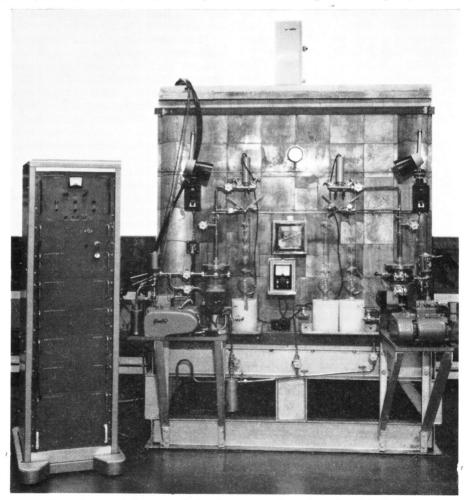
Fig. 1 General view of the new cell for the gas sampling of irradiated fuel elements using laser piercing techniques.
