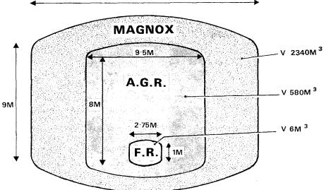
Fig. 5. Core dimensions of 600 MWE reactors.
