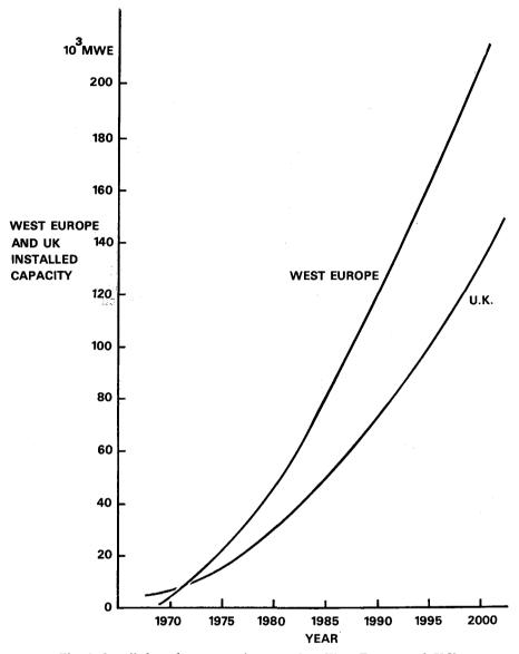
Fig. 1. Installed nuclear generating capacity—West Europe and U.K.
