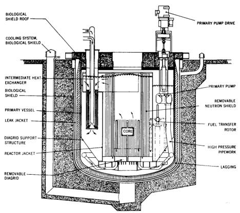
Fig. 7. The U.K. sodium cooled reactor.
