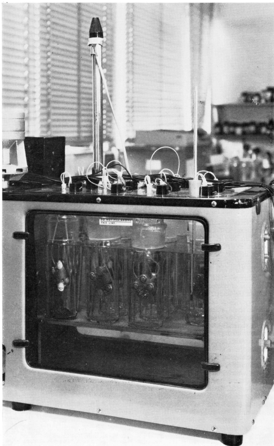
Fig. 2. Test tank, with cardiac pacemakers undergoing life tests in simulated body environment.
