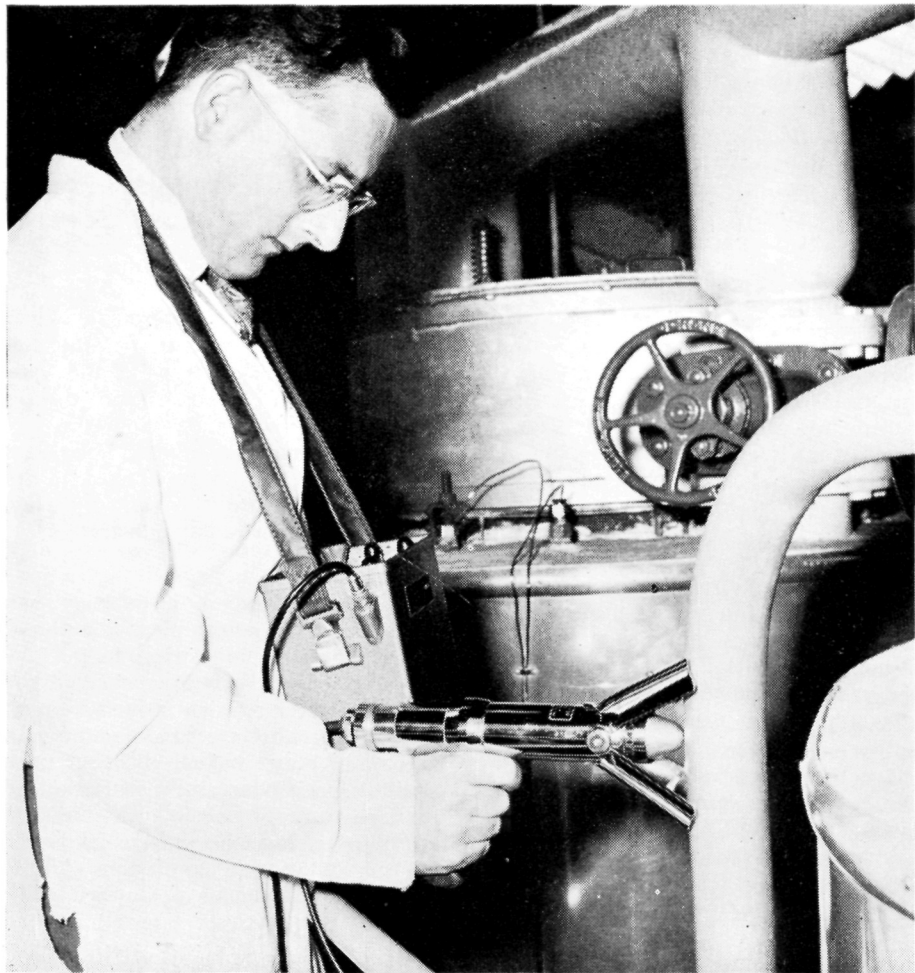
Fig. 2. A portable radioisotope thickness gauge for detecting internal corrosion in pipework.
