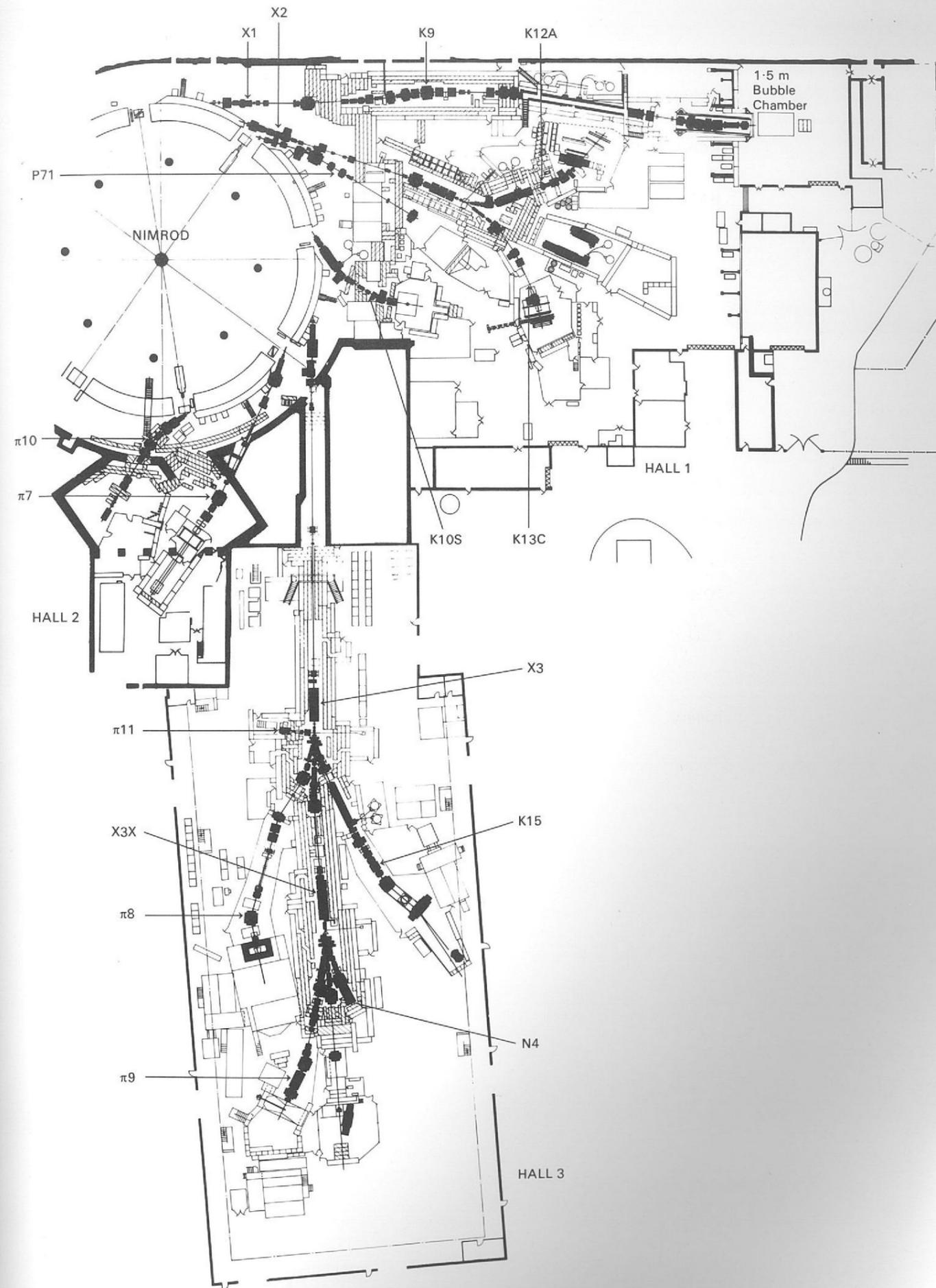
Figure 108. Beam lines in the Experimental Halls during 1972 (13482).
