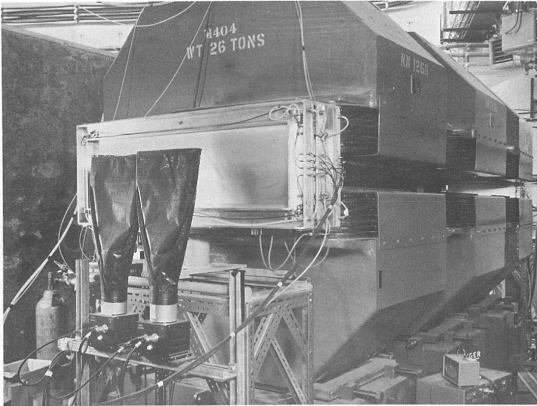
Figure 6. Acoustic spark chamber downstream from analysing magnets
