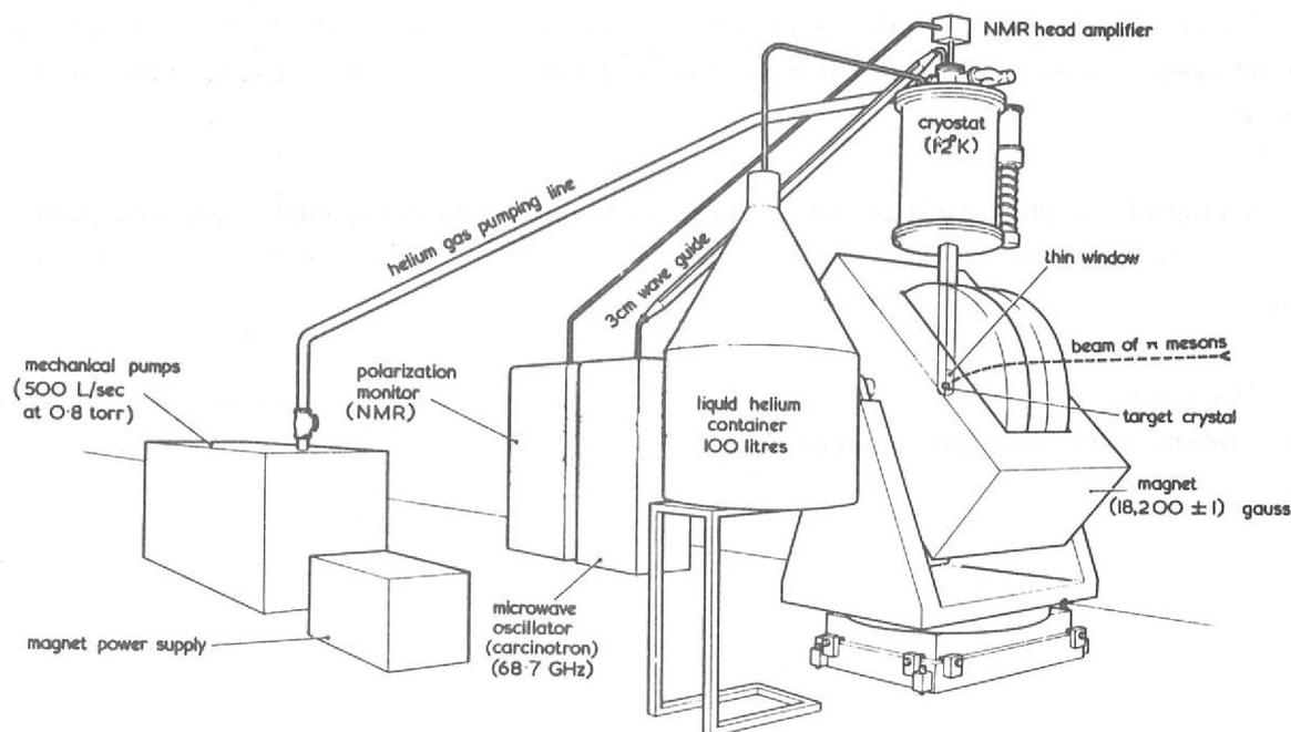
Figure 36. Schematic view of the first polarized target built at the Rutherford Laboratory in which the magnetic field was horizontal.
