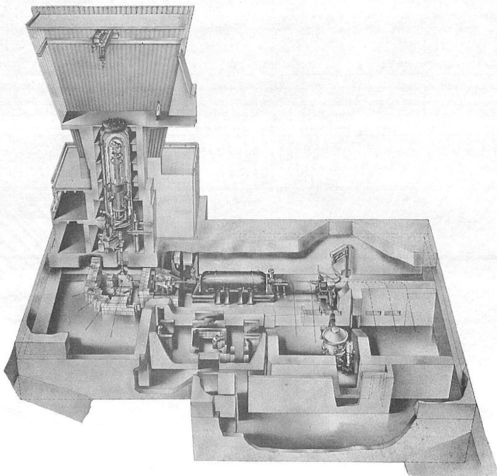
Figure 47. General arrangement of electrostatic generators at Oxford
