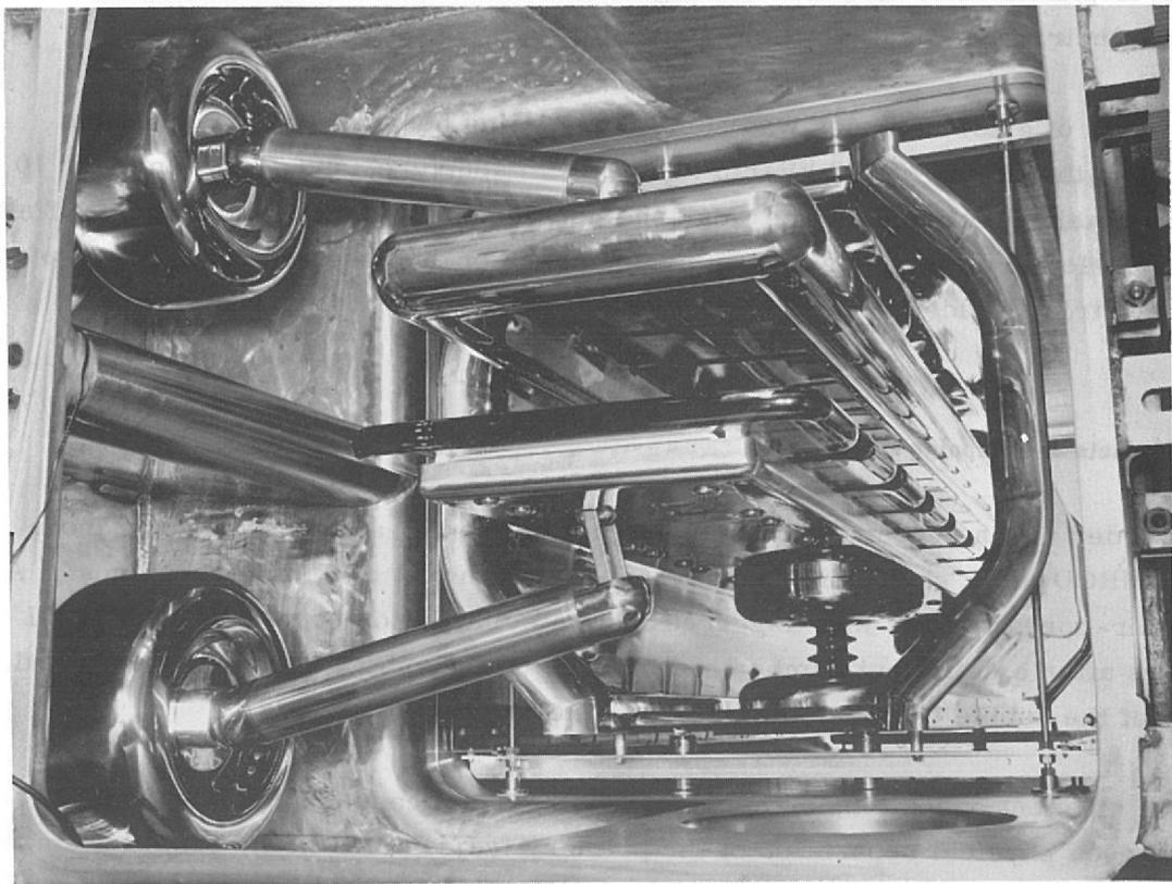
Figure 35. Internal view of electrostatic particle separator. A potential of 700 kilovolts is applied across the 10 cm gap between the stainless steel anode (top) and the heated glass cathode (bottom).
