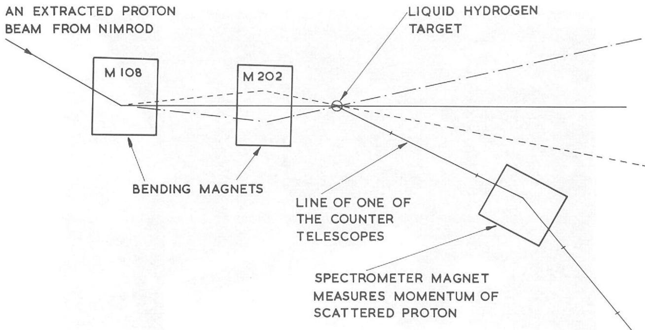
Figure 14. A schematic diagram of the Experimental Set Up for the Study of Nuclear Isobar Production in p/p collisions.
