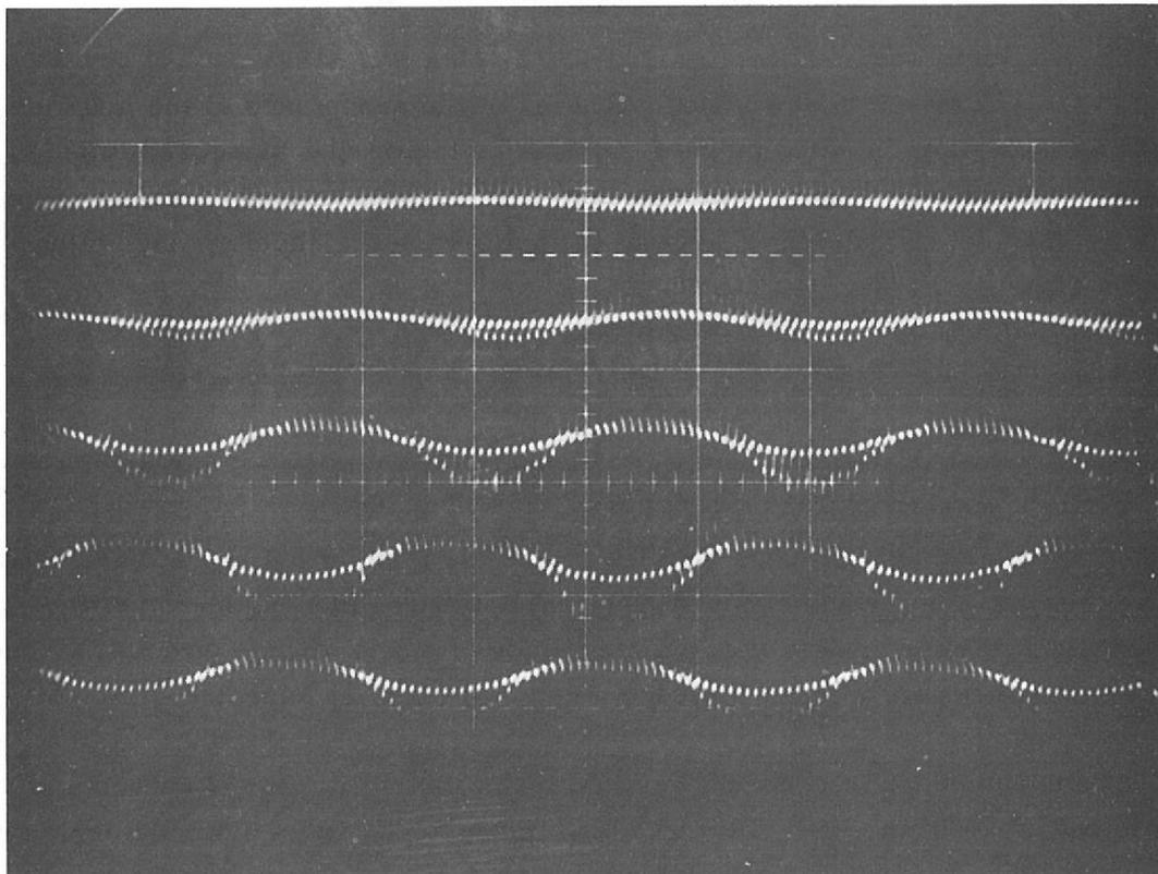
Figure 25. Build up of coherent vertical oscillations of the accelerated beam caused by the resistive wall instability. The successive traces are taken at 2 ms. intervals. Each small spike is the signal from one Nimrod bunch.
