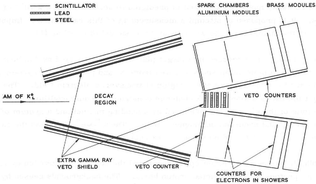
Figure 17. A schematic diagram of the apparatus used to detect the  $\pi^0 \pi^0$  of the  $K_L^0$
