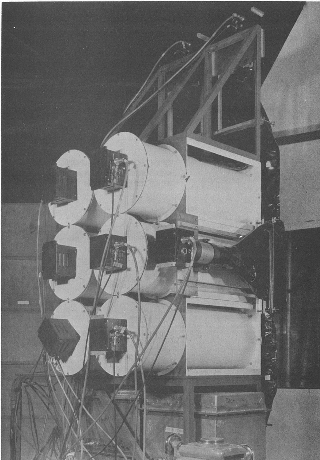
Figure 16. The Neutron Detectors Used in the Study of  $f^0$  Decays
