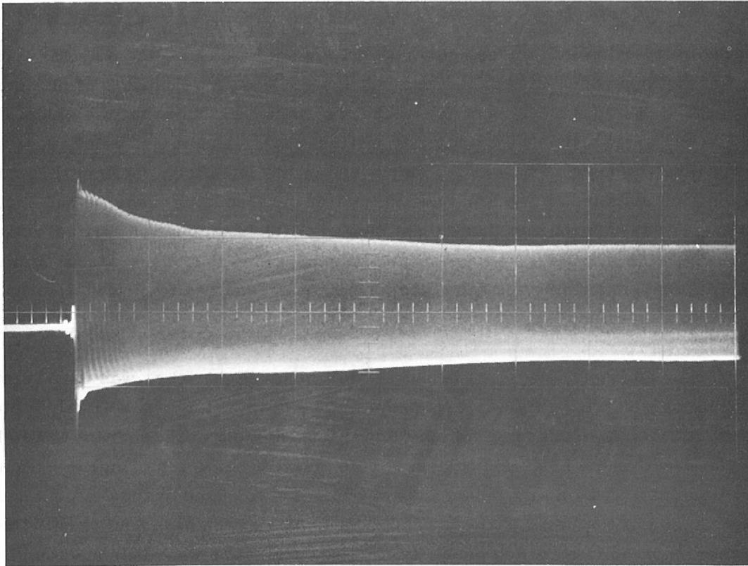
Figure 24. Signal from beam induction electrodes showing beam intensity loss at the beginning of the accelerating cycle. There is normally no loss of beam after the 18 ms. part of the cycle shown. The beam intensity at 18 ms. is about  $1.5 \times 10^{12}$  protons.
