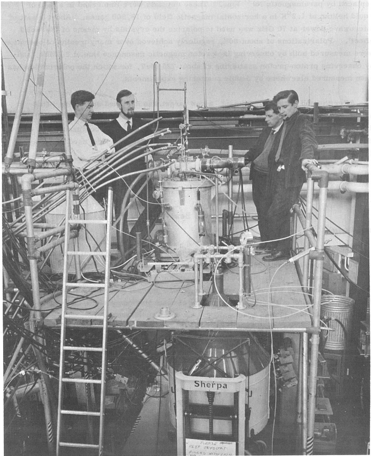
Figure 37. The First Rutherford Laboratory Polarised Proton Target
