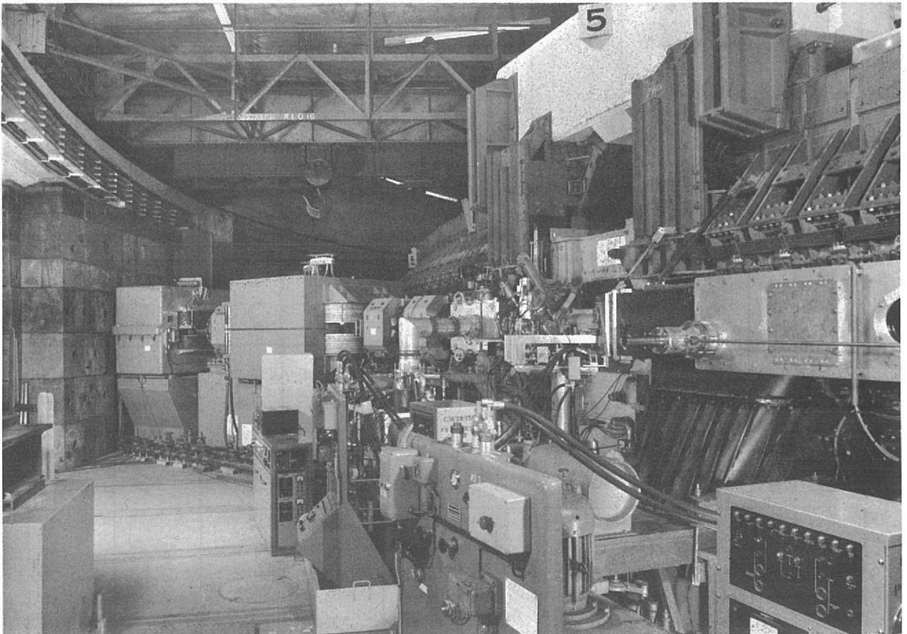
Figure 38. The magnet room end of the K1 beam line. Pions, kaons or protons are scattered from the target in the magnet at the right hand side of the photograph. After focussing and bending they pass through the steel shielding on the left hand side of the photograph to the first electrostatic separator buried in the shielding and thence to the experimental area.
