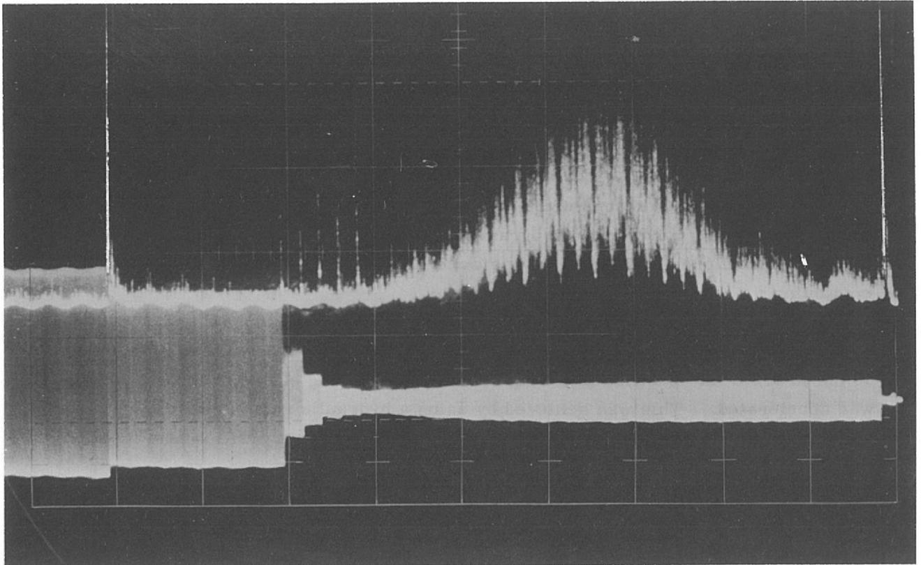
Figure 29. Sharing of accelerated beam. The upper trace shows a fast spill for a bubble chamber followed by a slow spill for one or two counter experiments followed by a second spill for the bubble chamber. The lower trace is the induction electrode signal showing beam intensity.
