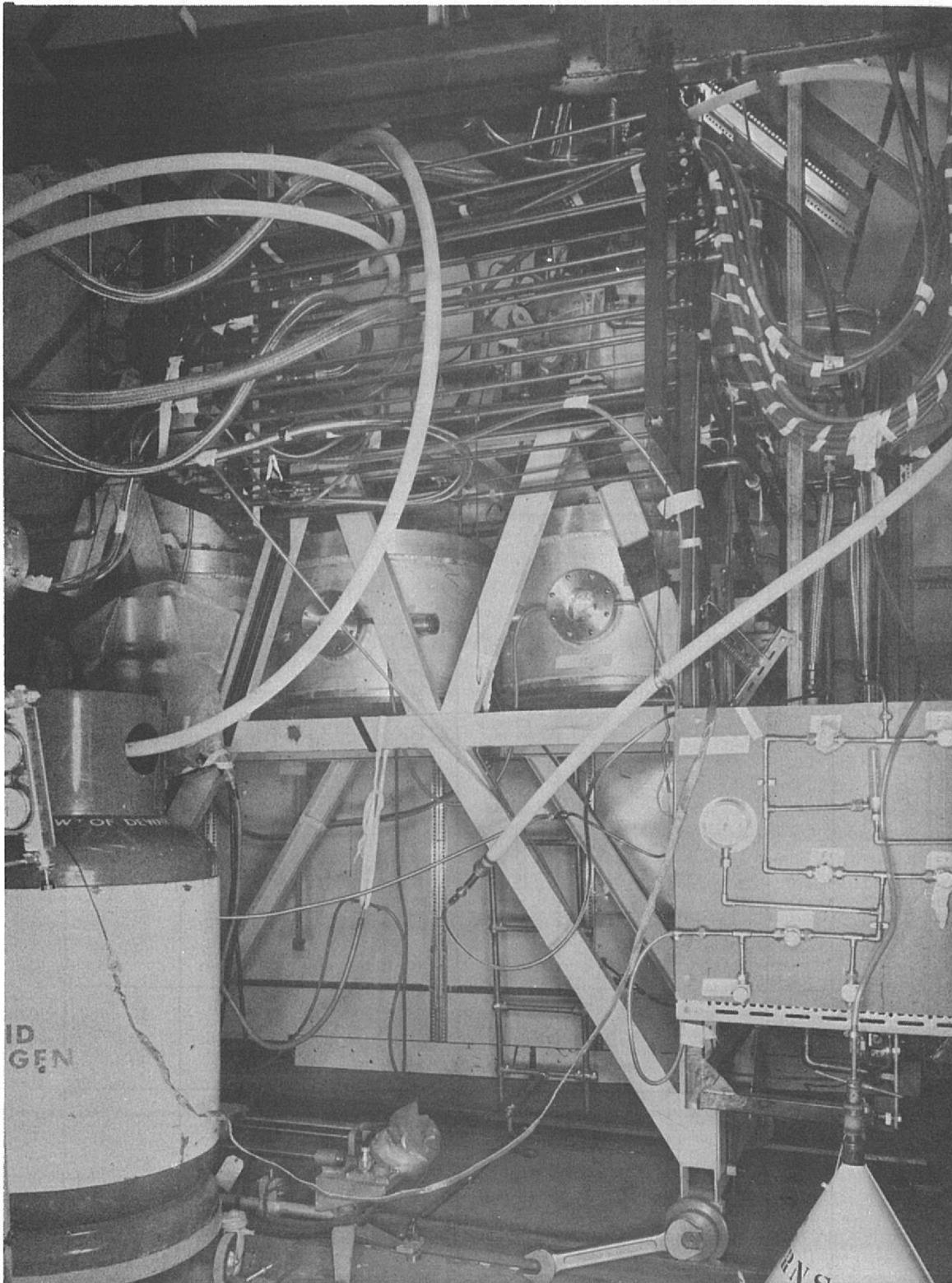
Figure 39. Target assembly for the P4 experiment. The left hand cylinder contains the liquid deuterium target, the centre cylinder is used for target empty runs and the right hand cylinder contains the liquid hydrogen target.
