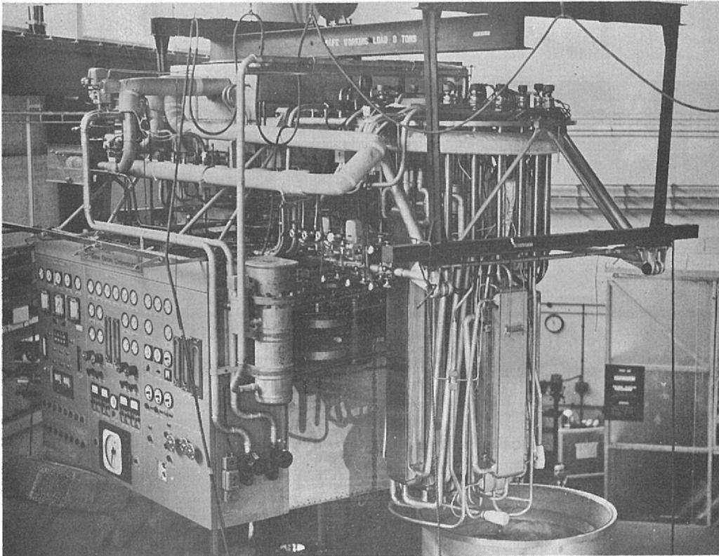
Figure 45. Refrigerator installation of the Liquid Helium Bubble Chamber
