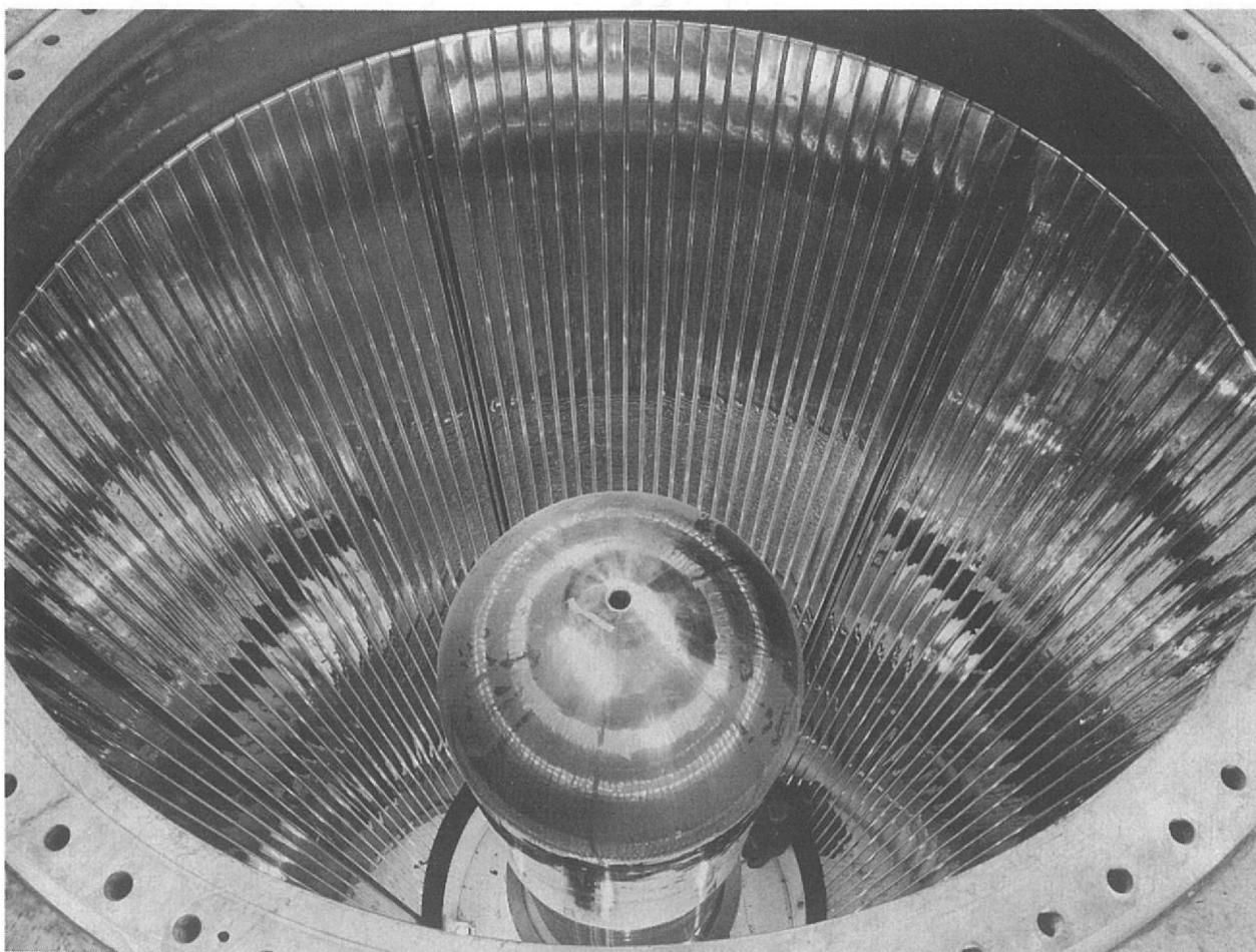
Figure 46. Top view of the Injector of the Oxford Electrostatic Generator
