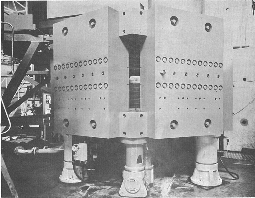
Figure 44. Magnet of the Liquid Helium Bubble Chamber
