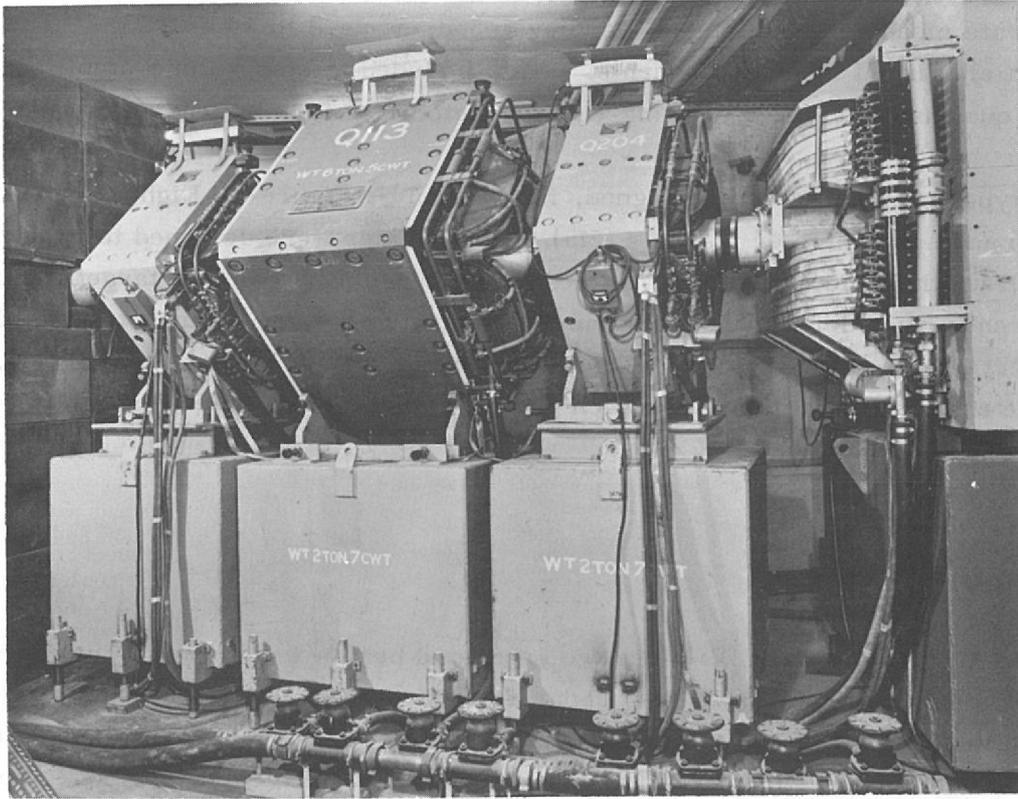
Figure 34. A section of beam line showing standard quadrupoles and part of a bending magnet
