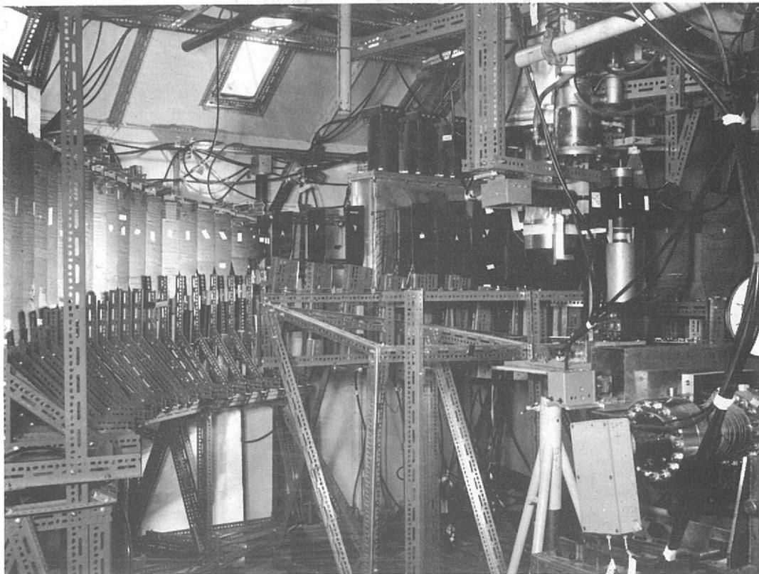
Figure 7. Array of scintillation counters for the study of pion/proton scattering
