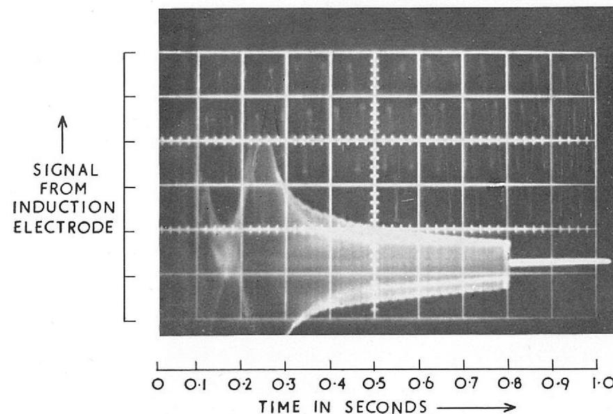
The trace shows the signal from an induction electrode: a hollow metal box through which the proton beam passes on each circuit of the accelerator. Each circulating proton on passing through the electrode induces a charge on it, so a circulating bunch of protons is detected by an oscilloscope connected to the electrode, as a voltage pulse whose area is proportional to the circulating charge.
