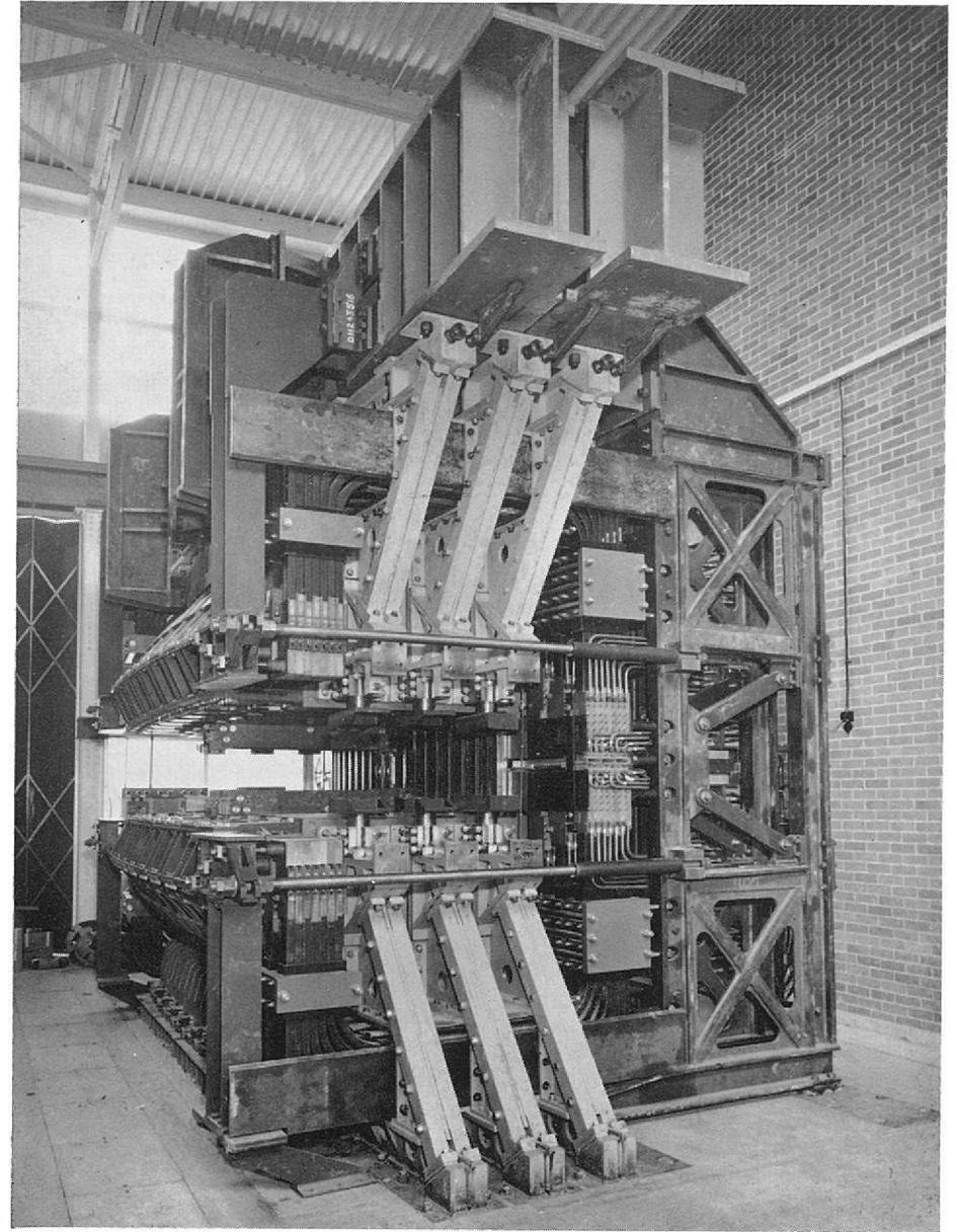
Full scale model of a section of the Nimrod magnet built to test various features of the design.
