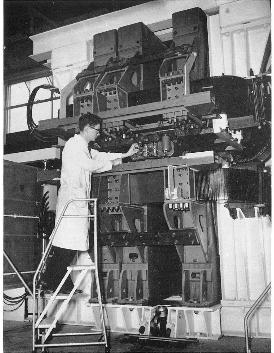
Testing rig for measuring magnetic properties of Nimrod magnet sectors
