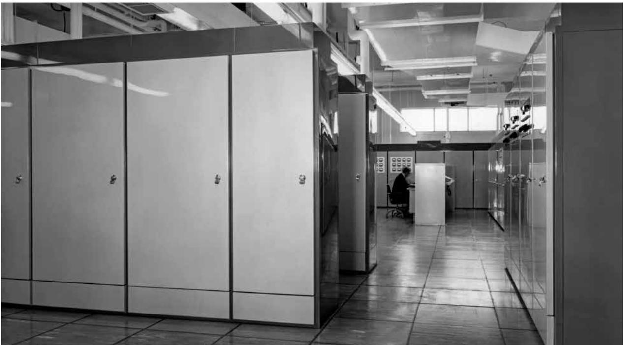
The Atlas machine room seen from the other end of the room. The power supply and switching units are on the right of the picture; core store cabinets are on the left.
