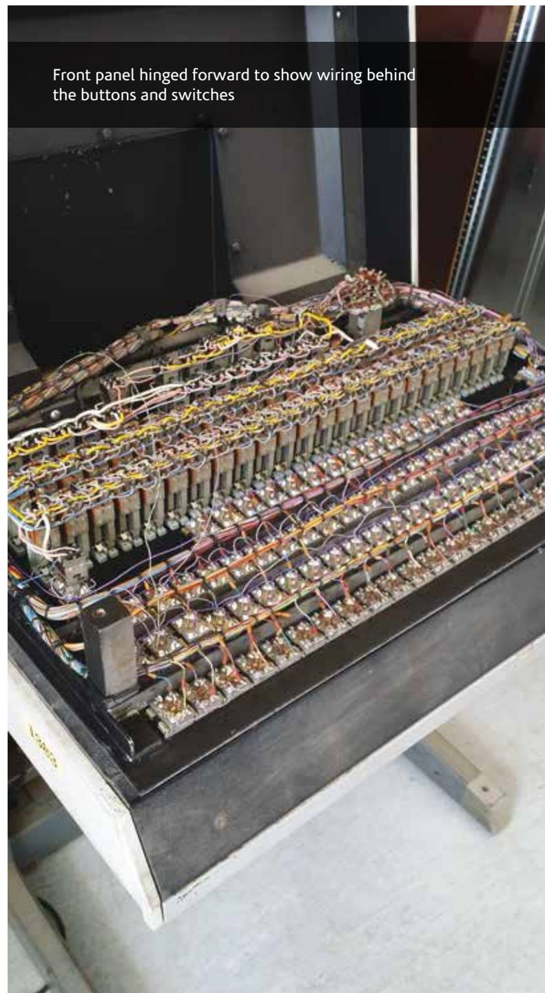
Front panel hinged forward to show wiring behind the buttons and switches
