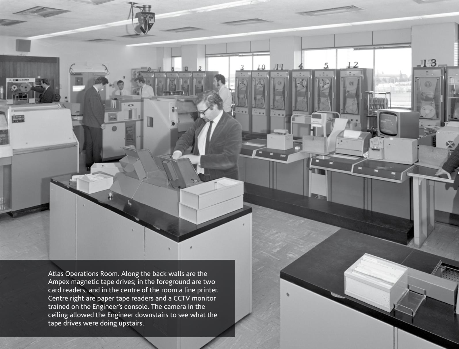
Atlas Operations Room. Along the back walls are the Ampex magnetic tape drives; in the foreground are two card readers, and in the centre of the room a line printer. Centre right are paper tape readers and a CCTV monitor trained on the Engineer's console. The camera in the ceiling allowed the Engineer downstairs to see what the tape drives were doing upstairs.
