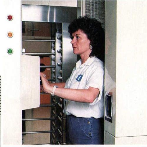
Monitoring the whole body for radioactive contamination takes only a few seconds
