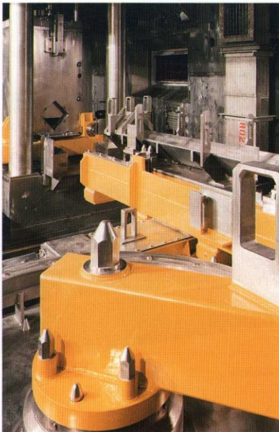
The hydraulically operated shear machine in THORP is designed to cut fuel into pieces.
