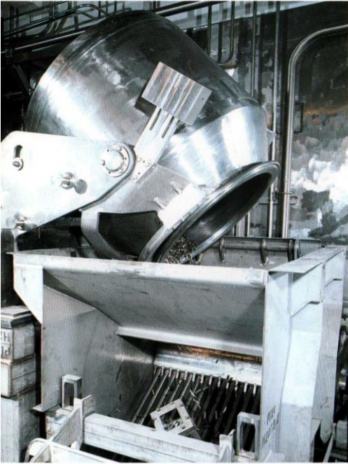
Solid intermediate-level waste from THORP is fed in controlled quantities into a drum before being encapsulated in concrete.
