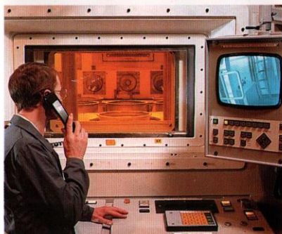
TOP A waste drum is posted into the cell from the roof area.
