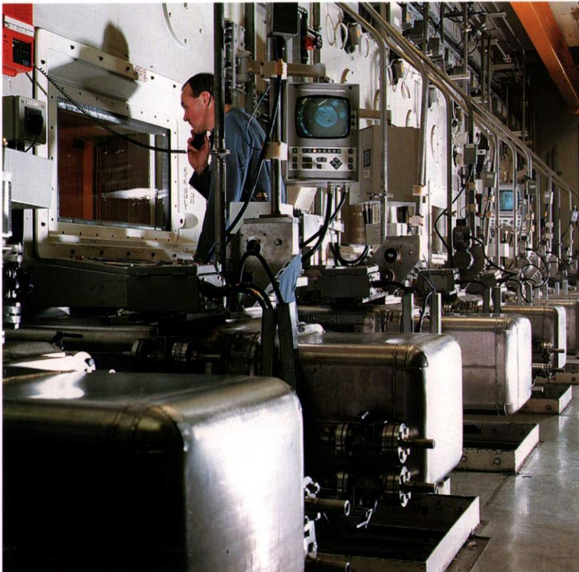
ABOVE A total of ten capping grout stations prevent a backlog of drums from building up.
