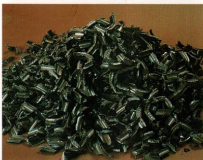
TOP Magnox cladding is removed in the Fuel Handling Plant.
