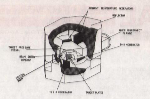
Because the experiments measure the neutron energies by time of flight techniques the moderators must be small (typical volume 0.5 1). Neutrons which might have missed such small moderators are scattered back into the by a Reflector made of Beryllium rods cooled by heavy water. This results in neutron beams which are three times greater than they would be without the reflector.
