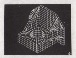
The structure is divided up into a number of elements (a process known as meshing or discretisation), where each element defines the stiffness of the structure at that point and is dependent on the geometry at that location and on the material used for the structure. In this way the stiffness of the whole structure is described mathematically and can be stored in a computer.
