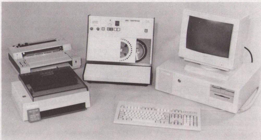
PC controlling a particle sizer which uses centrifugal sedimentation of samples dispersed in a liquid.
