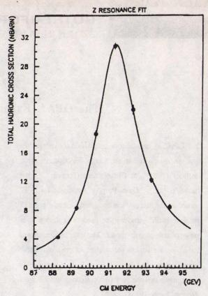
operated, and the curve shown above has been obtained by varying the LEP energy. It is possible to deduce the number of different types of neutrino which exist from the shape of this curve. This measurement is important because it is closely related to the total number of fundamental particles from which the universe is constructed.
