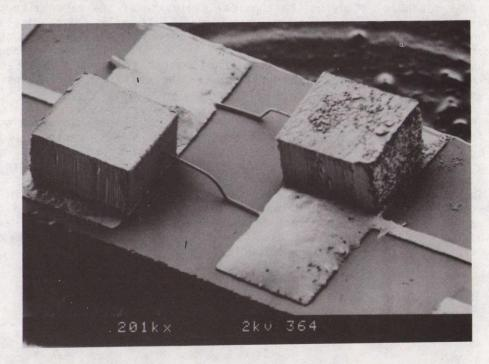
Scanning electron micrograph (magnification 200x) of two diode chips mounted on a quartz printed circuit board in an antiparallel configuration. The diameter of each of the two 'whisker' wires is 5 microns. This is six times less than the diameter of a human hair.
